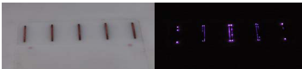
Figure 6.2. Ionization plate setup and corona discharge at a potential difference of 20 kV.
