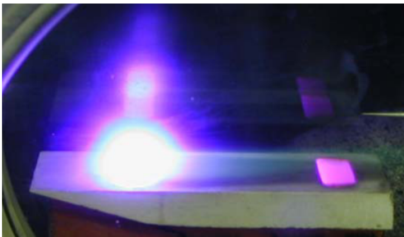
Figure 3.8. A DC voltage discharge between two electrodes at freestream conditions of M = 5.15 and p = 0.59 torr. The applied voltage is 880–920 V at a current of 50 mA. The addition of a magnetic field significantly affects the plasma and creates a virtual hypersonic leading edge strake (from [7]).
