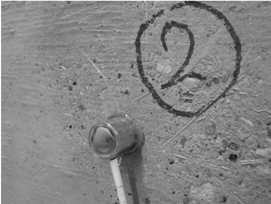
Figure 3-13 Typical AE sensor bonded to test specimen
