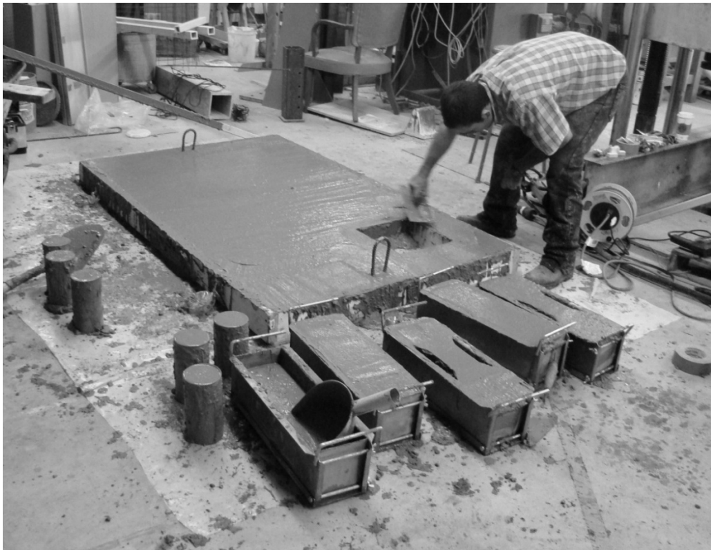
Figure 2-1 Casting of large-scale specimens and ASTM beams and cylinders
