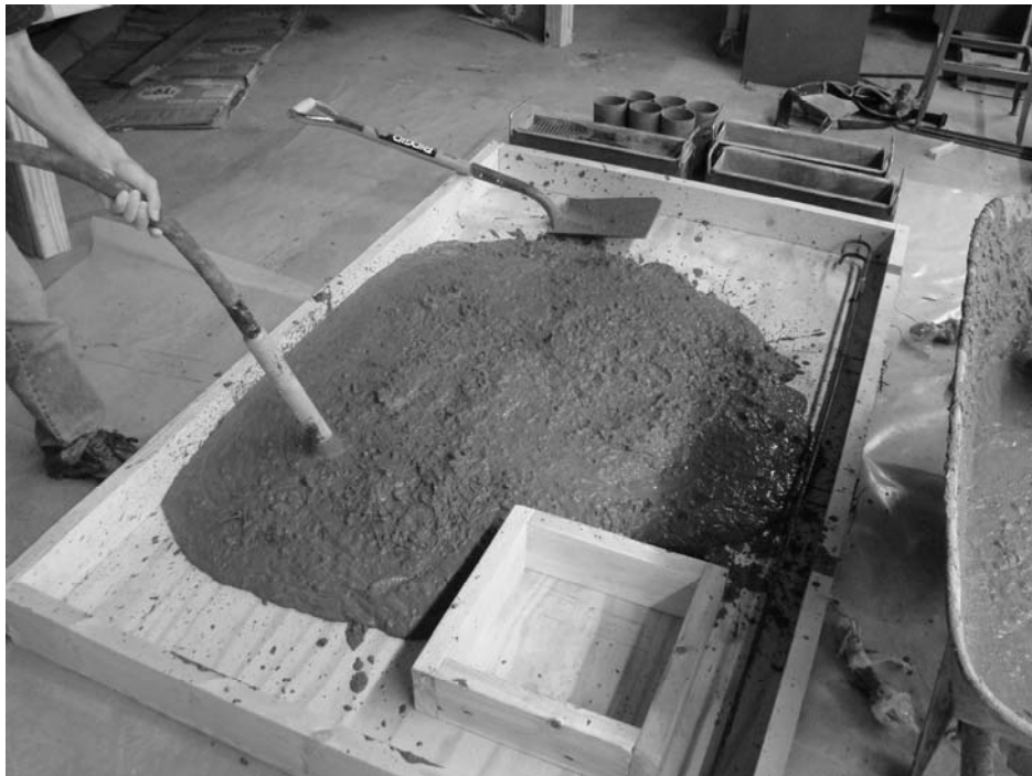
Figure 3-29 SFRC test specimen during placing and consolidation of plastic concrete
