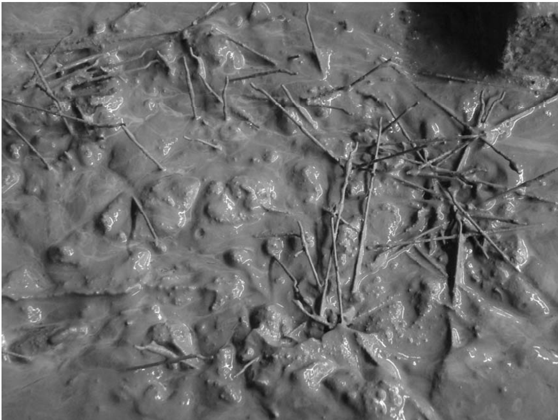
Figure 3-30 Close-up of plastic SFRC during casting
