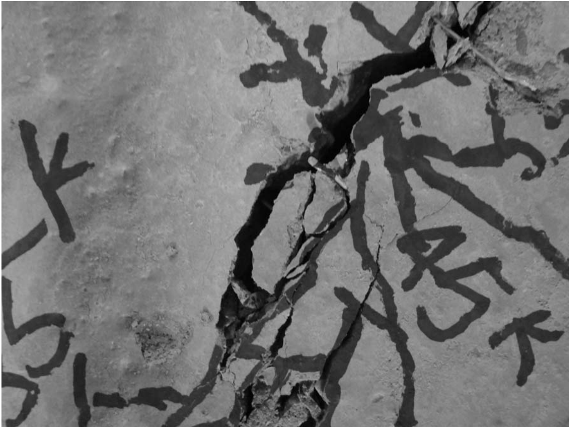
Figure 3-36 Steel fibers pulling out of the diagonal crack at ultimate load (front face)
