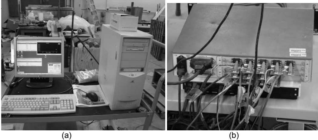
Figure 3-8 Data acquisition system (a) and scanner box (b)
