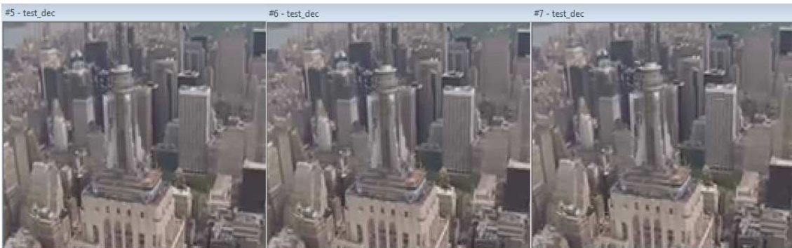
Figure 6.8: Frame# 5 is the decoded frame. Here Frame# 6 successfully copied lost information from Frame 5 by copy algorithm; Frame #7 is degraded (Because Frame#7 is reconstructed by collecting the information from previous reference frames).
