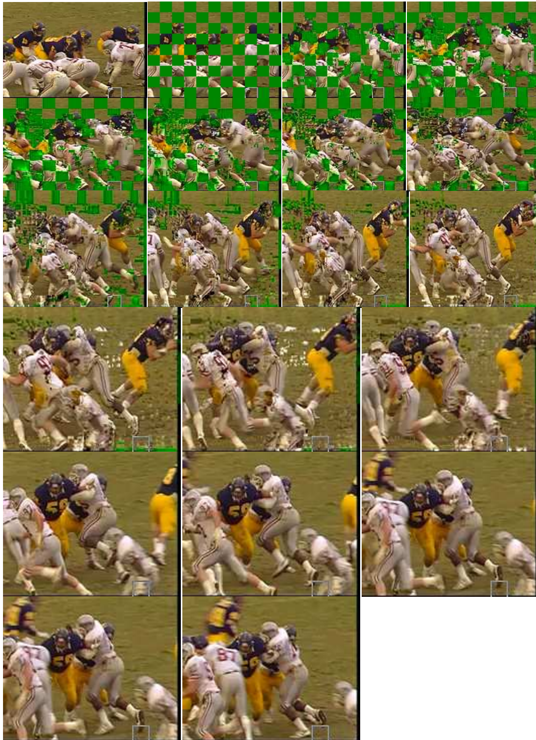
Figure 6.11: Frame#1 to frame#20 of distorted video sequence due to the packet loss during transmission of bit stream in an error prone wireless medium.
