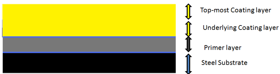
Figure 4.1 Schematic for samples with all additives in a blend Part-I and Blend Series
