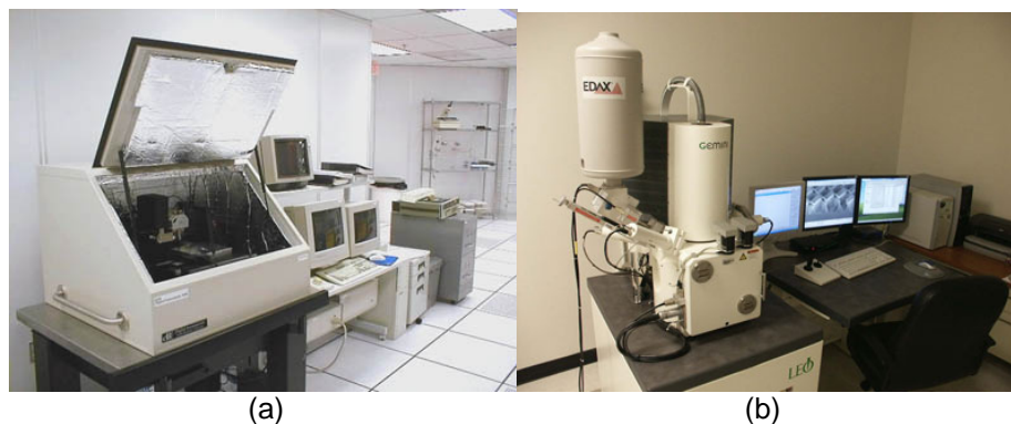
Figure 3.8 (a) Veeco Dimension 5000 AFM (Tapping Mode, contact mode, MFM); (b) ZEISS Supra 55 VP SEM
