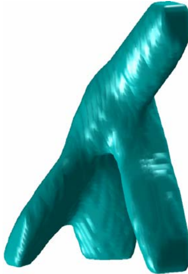
Figure 3.18 Coarse mesh with multiple Loads: Solution using Perturbation and Sequential Linear Programming. 30 minutes were required to run 600 sequential iterations.
