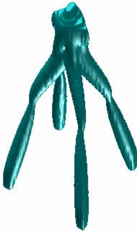
Figure 3.9 Stool: Solution using Particle Swarm Optimization with parallel processing. Cluster consists of Dell PowerEdge 1950 dual quad core 2.33GHz Intel EM64T Xeon processors with 16GB of memory each. 25 hours were required to run 600 particle swarm iterations with population size of 128 per iteration (76800 objective evaluations).
