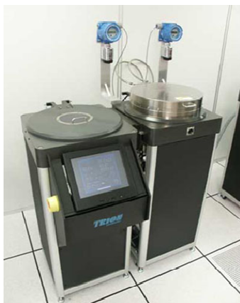
Figure 2.2 TRION ORION II PECVD/LPCVD System, NANOFAB, UTA. [17]
