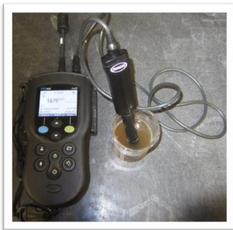
Figure 3.8 Conductivity Probe and Meter
