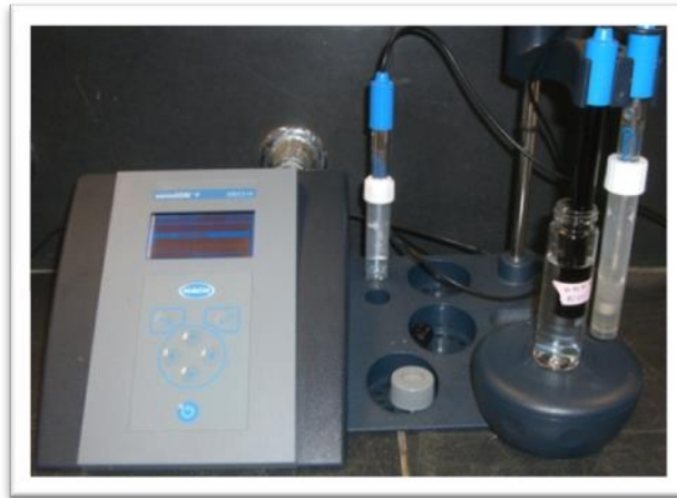
Figure 3.10 Chloride Probe and Meter Setup
