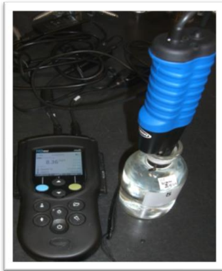
Figure 3.6: Dissolved Oxygen Probe and Meter
