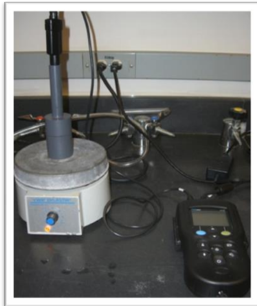
Figure 3.11 Ammonia-Nitrogen Probe and Meter
