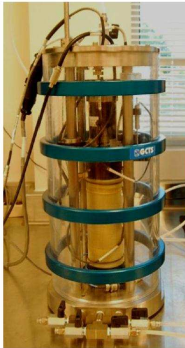
Figure 3-4 RC Main cell of the Proximator-based RC
