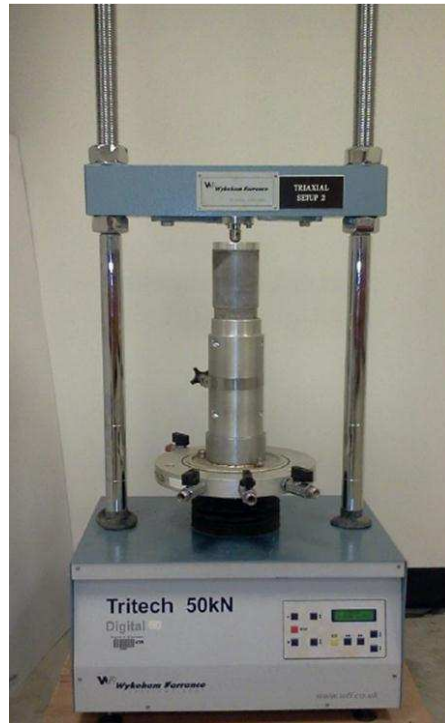
Figure 3-9 Triaxial loading frame used to compact cylindrical specimens
