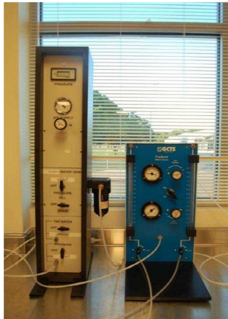
Figure 3-7 Panels for pressure control
