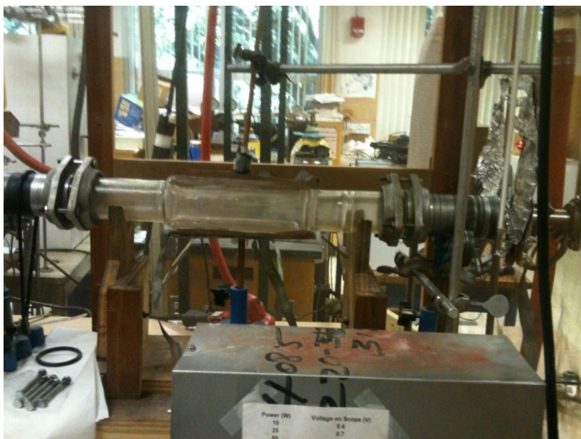
Figure 2-5 Picture of the rotary plasma reactor with electrodes outside of the glass reactor
