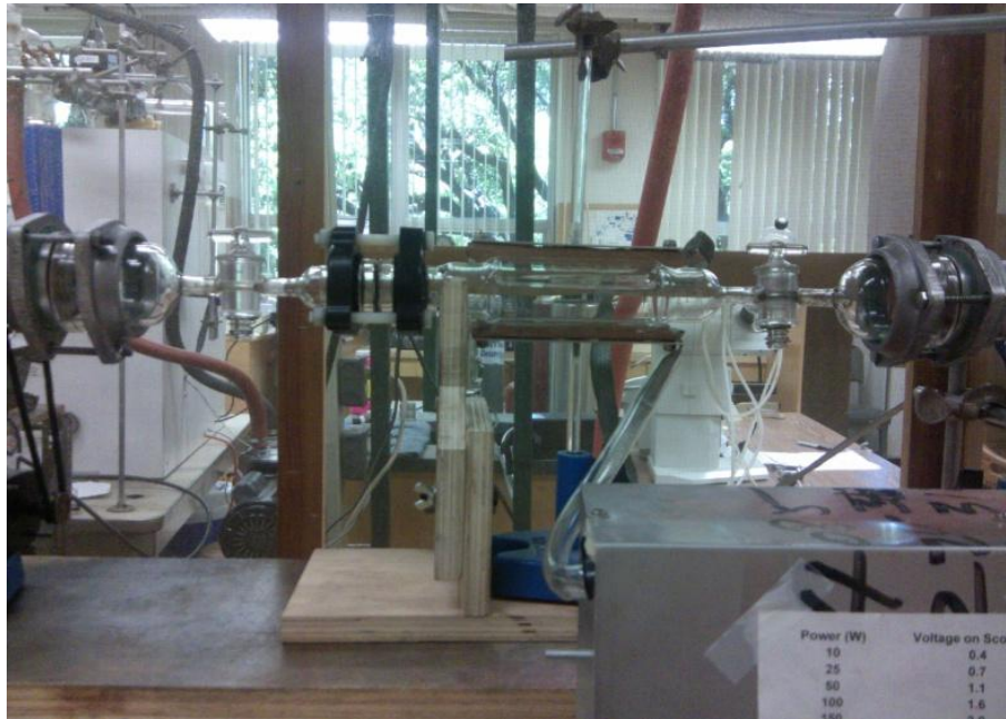
Figure 2-6 the newly designed glass reactor for plasma treatment of SmCo powders
