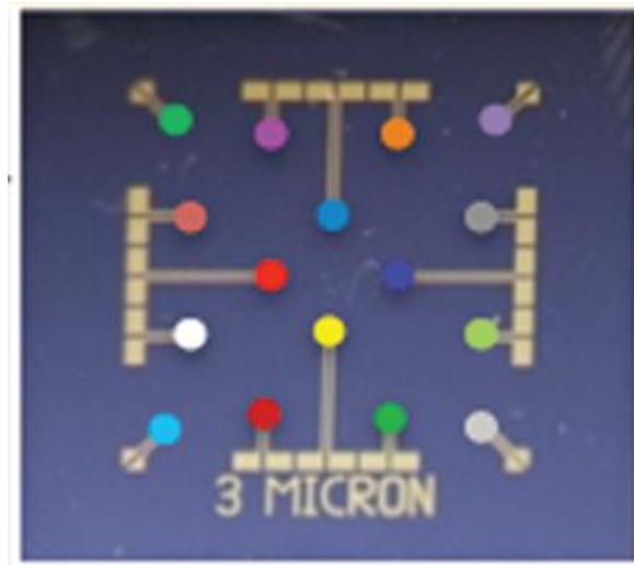
Figure 2-6 Porphyrin-Functionalized Single-Walled Carbon Nanotube Chemiresistive Sensor Arrays for VOCs layout.
