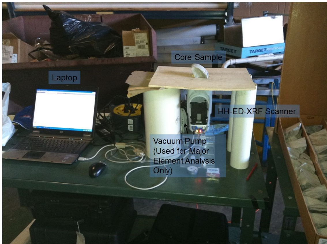
Figure 5. Setup of HH-ED-XRF showing laptop for collecting data from the scanner, a core sample resting on the nose of the instrument, the scanner (BEG-SD3), and the vacuum pump (partially obscured by a PVC pipe) scanning a core sample for major element analysis.
