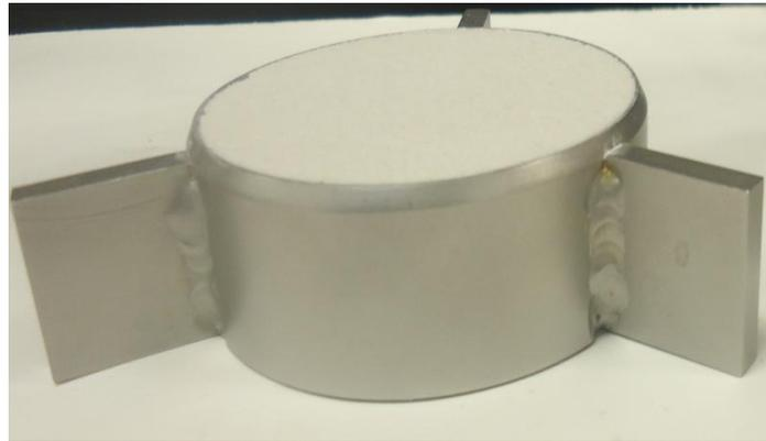
Figure 4.2 Silty sand specimen cut to fit into the retaining ring
