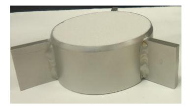
Figure 4.2 Silty sand specimen cut to fit into the retaining ring
