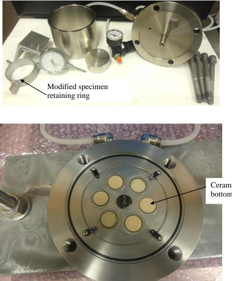
Ceramic disk on top of bottom plate.
