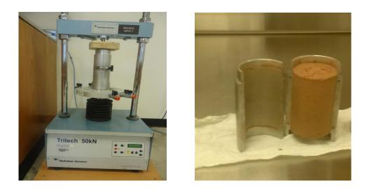
Figure 4.1 Triaxial compaction frame and typical sample after compaction
