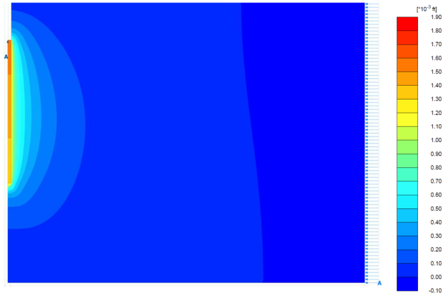
Figure 4.32: Example of the deformation of the soil nail and surrounding soil in PLAXIS 2D.
