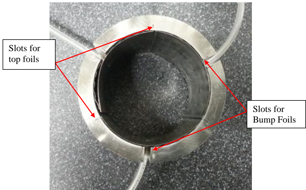
Figure 3-3 Current Hybrid Air Foil Bearing assembly
