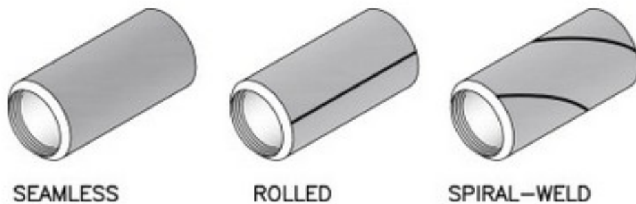
Figure 1.4 Different Types of Steel Pipes: Seamless, Rolled and Spiral Weld (Parisher & Rhea, 2012)
