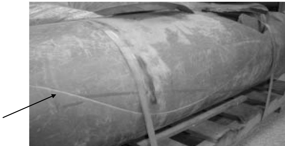
Figure 2.4: Noticeable Crack in PVC Pipe (Burn, et al., 2005)
