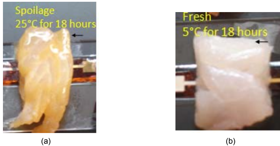
Figure 5.1 The test of our freshness indicator in different temperature at (a) 5°C and (b) 25°C.
