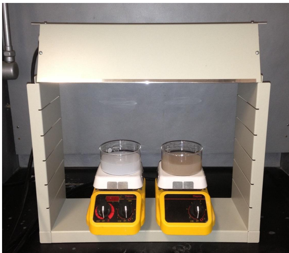
Figure 2.6 Configuration of Photo-Reactors Equipped with UV Lamps
