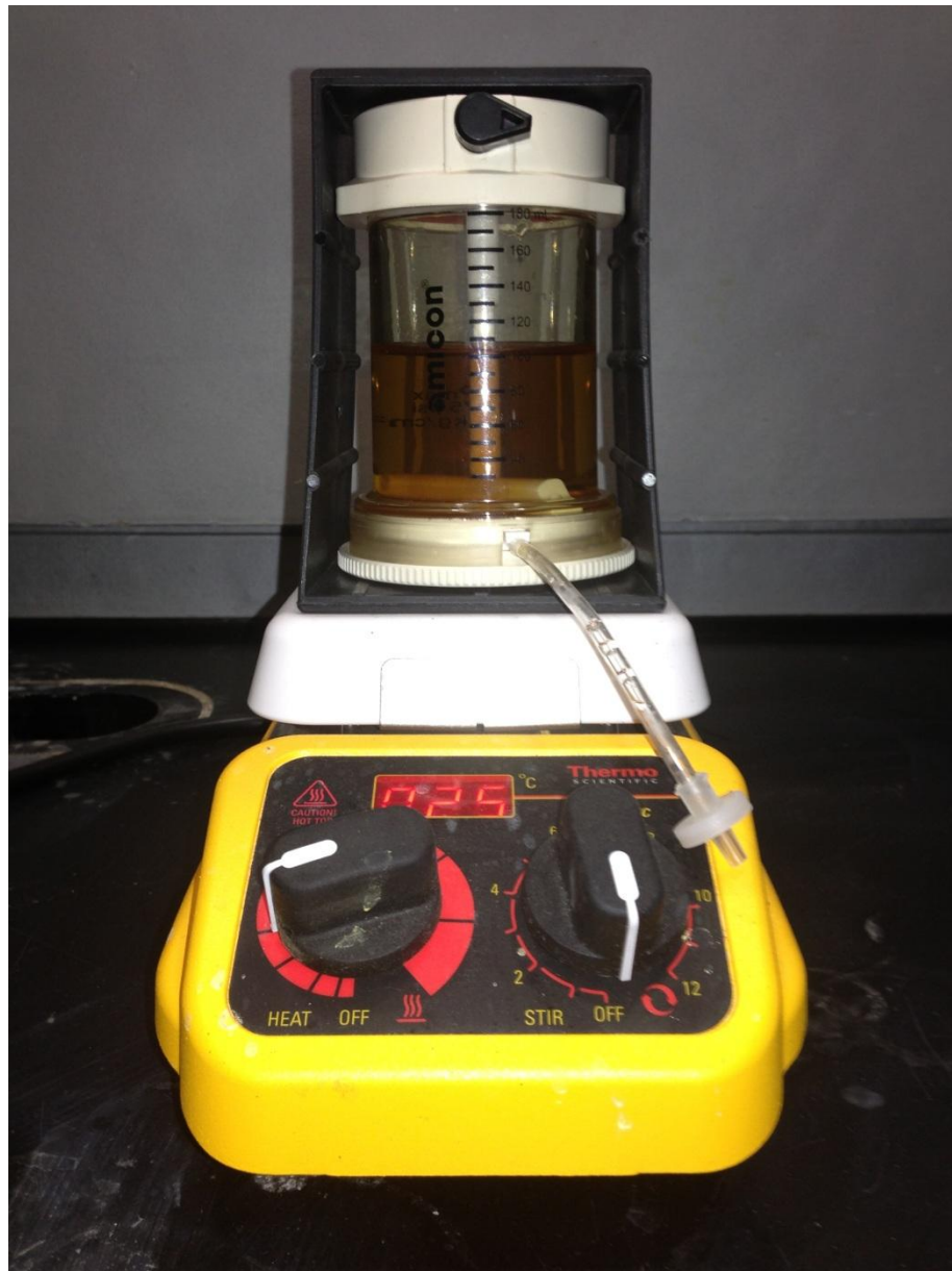
Figure 3.15 Ultrafiltration of HA using Pressure Driven Filtration Unit Equipped with Magnetic Stirrer
