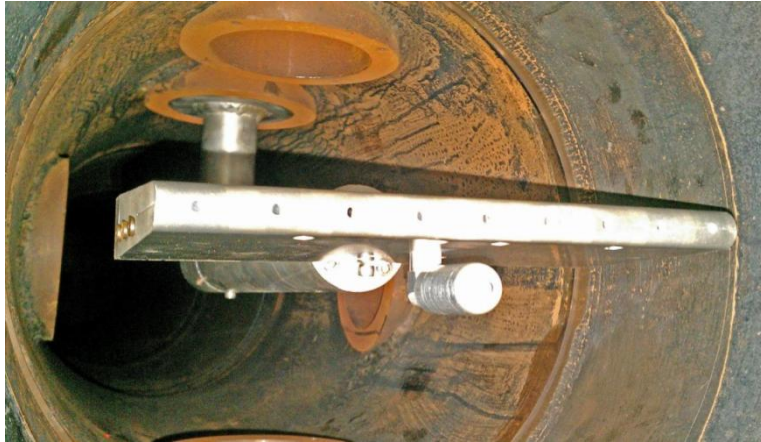
Figure 2.8 Sting and pressure rake as mounted in test section; Leamon [4].
