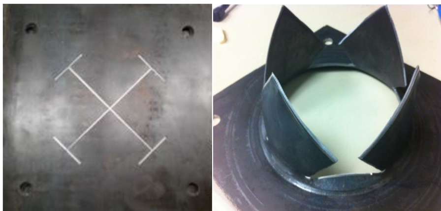
Figure 2.2 Primary diaphragms scored and after successful test
