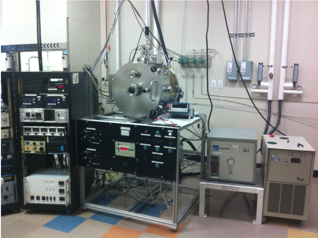
Figure 3-4 Lab-Built PVD reactive magnetron sputtering system in Surface and Nano Engineering Laboratory
