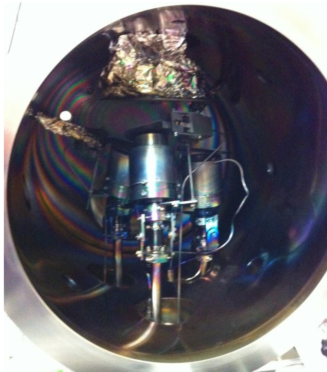
Figure 3-5 Lab-Built PVD Reactive Magnetron Sputtering System in Surface and Nano Engineering Laboratory
