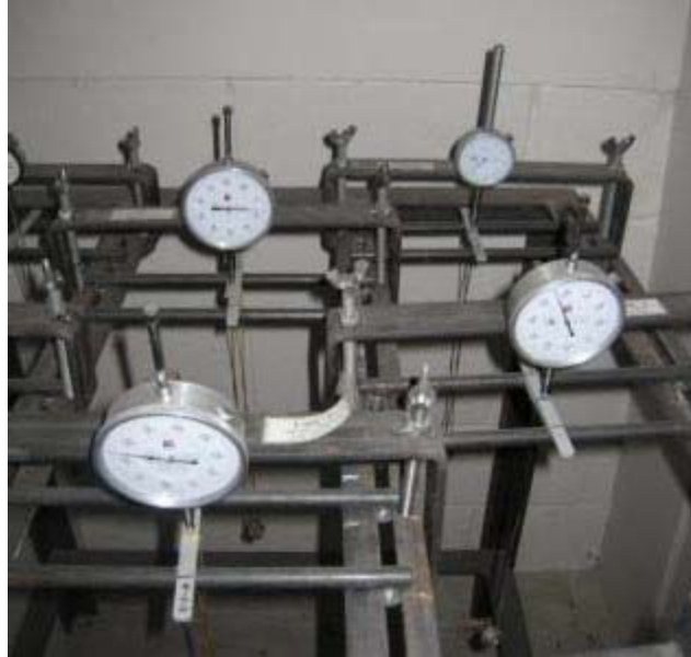
Figure 3.3- Test Apparatus and Specimens for Flexural Test
