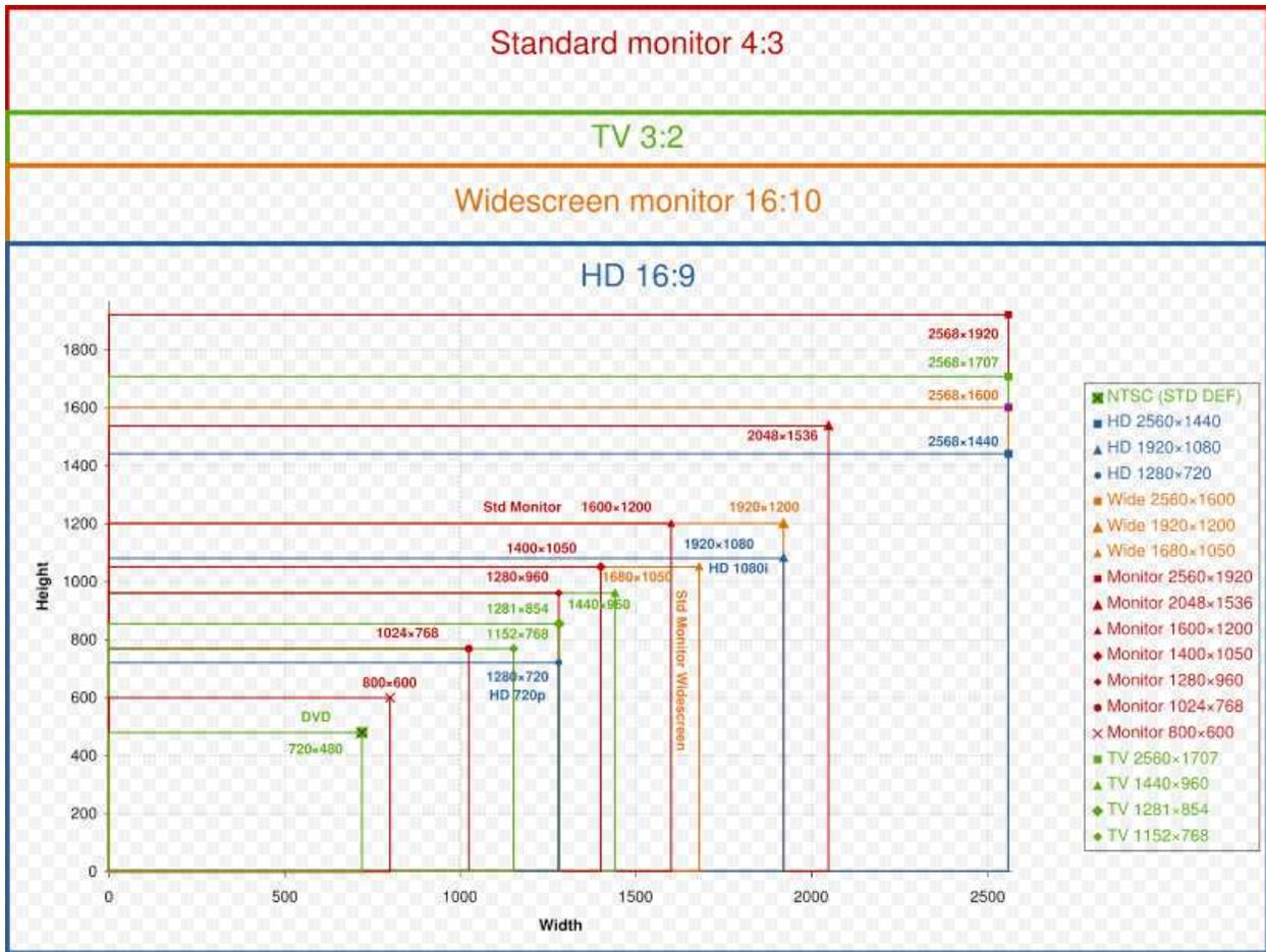
Figure 2.4: Various screen resolutions at users end [27].
