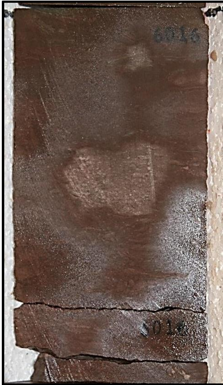
Figure 21: Core photograph of red/brown silty dolomite with wispy laminations indicating oxidizing conditions (6016').
