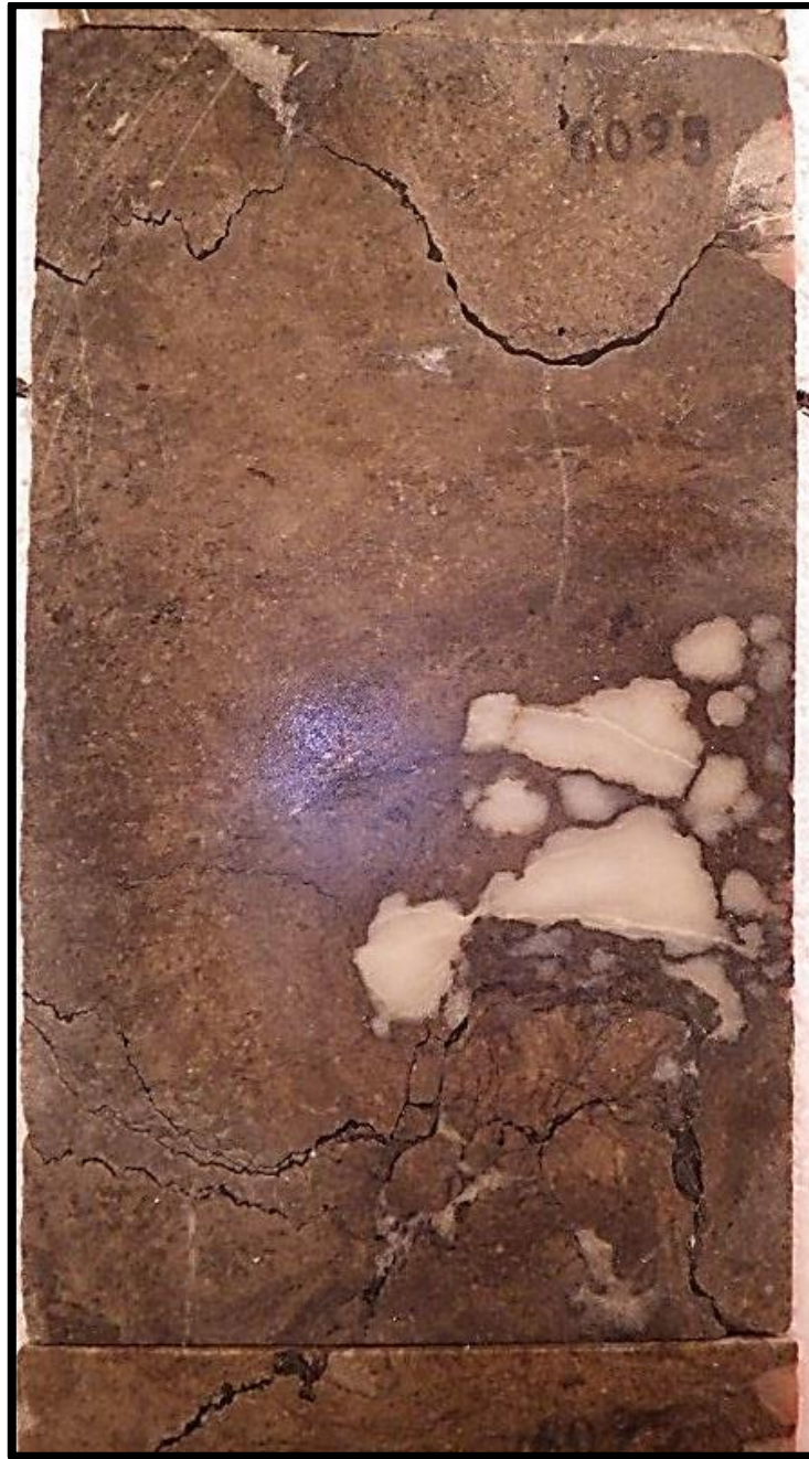
Figure 14: Core photograph of recrystallized mudstone/wackestone facies from the bottom of sub-interval C displaying well developed stylolites.
