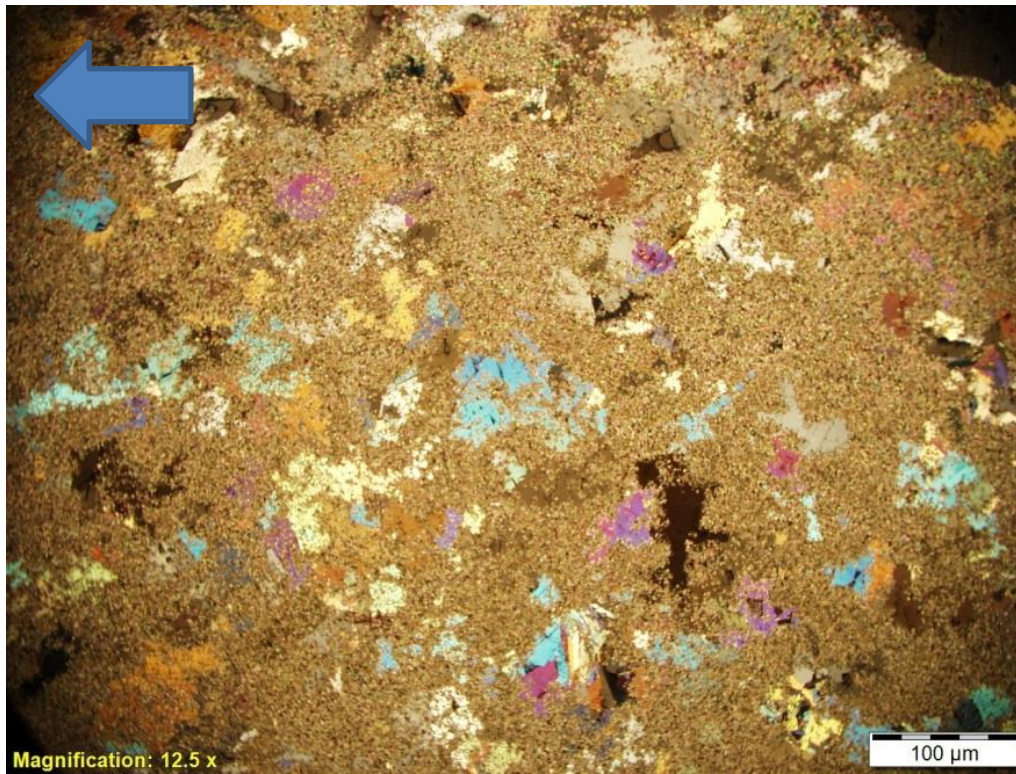
Figure 37: Photomicrograph of pore filling anhydrite (high birefringence colors) in a dolomite matrix. The anhydrite occludes much of the secondary pore space. Sample G2-6090. 12.5x CPL. Arrow indicates stratigraphically up.
