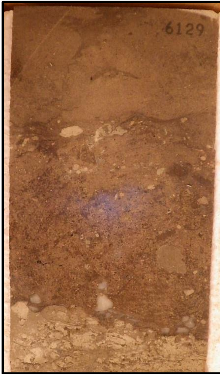
Figure 10: Core photograph of rudstone from depth 6129'. Notice the mud intraclasts probably transported from nearby environments.
