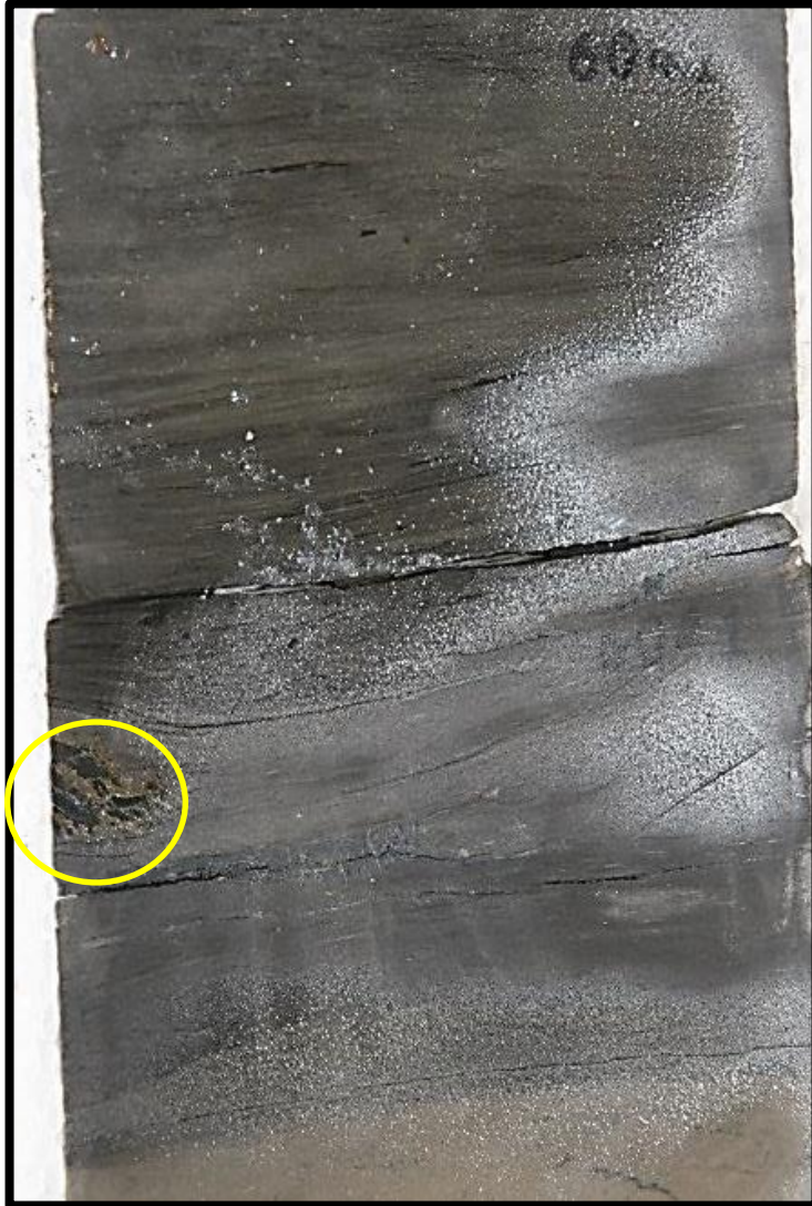
Figure 17: Core photograph of pyrite nodule in organic rich shaley mudstone. Pyrite nodule is an indication of anoxic conditions, like a result of lagoonal starvation where algal mats could grow but carbonate production is limited.
