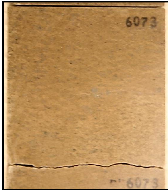
Figure 60: Core photograph of homogenous lithology. Sample E2-6073 which contains very similar SEM and whole-core helium porosity values.
