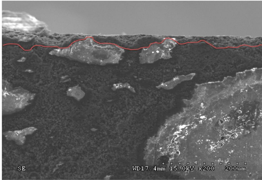
Figure 5-39: The SEM micrograph showing the formation of a softened area at a 17mm radius.
