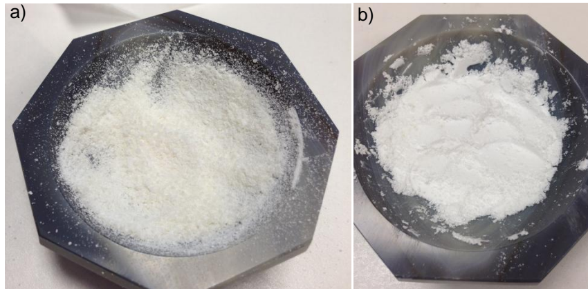
Figure 4-2: The appearance of a) erucamide and b) silica after being crushed by the pestle.
