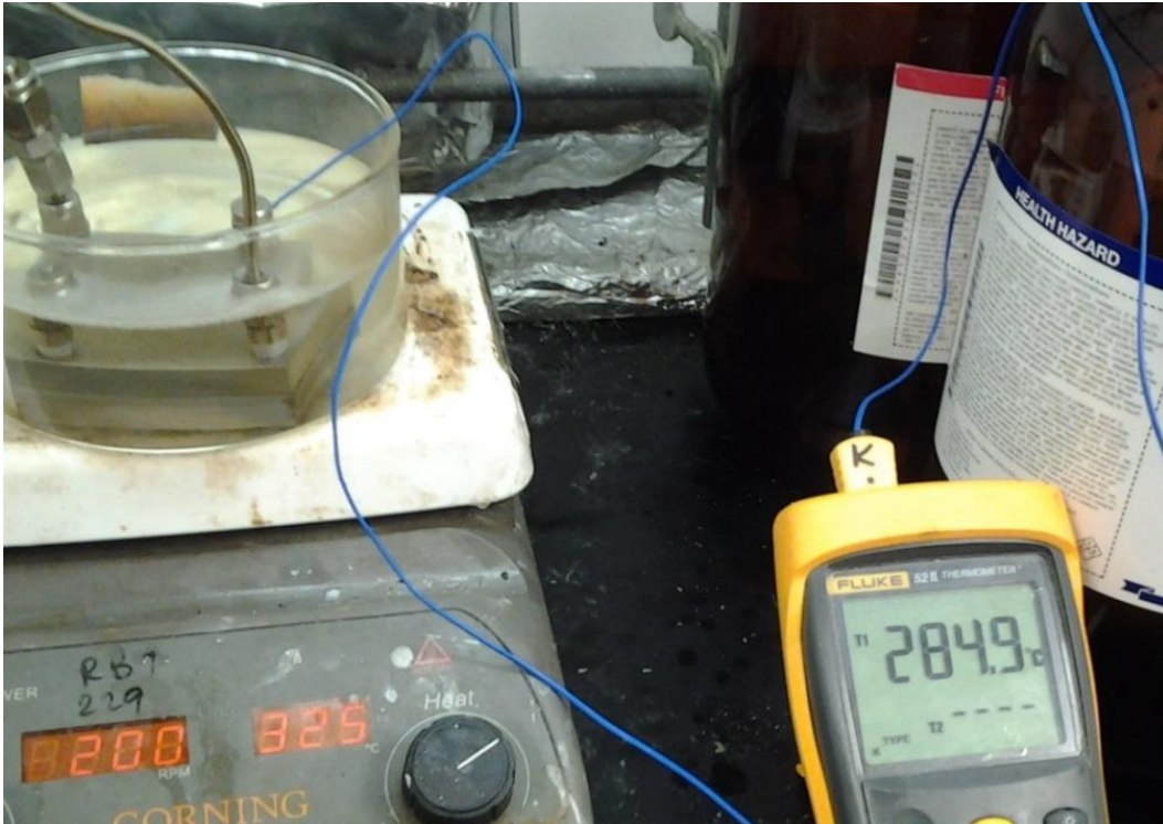
Figure 5-1 Leak-testing a microreactor in silicone oil
