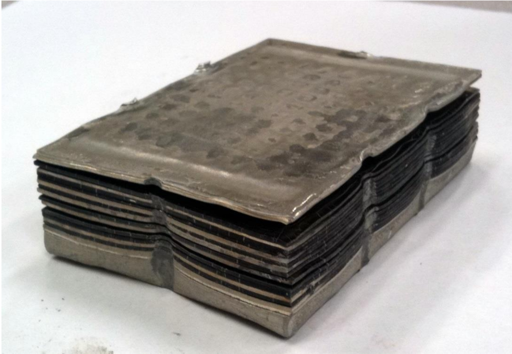
Figure 5-10 Aluminum oxide prevents diffusion bonding
