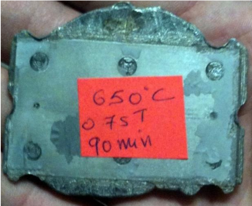
Figure 5-5 A specimen that received too much heat and force
