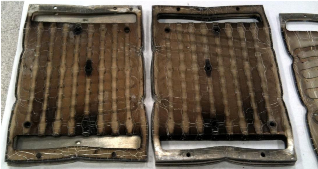
Figure 5-11 Aluminum oxide cracks as interior aluminum alloy deforms
