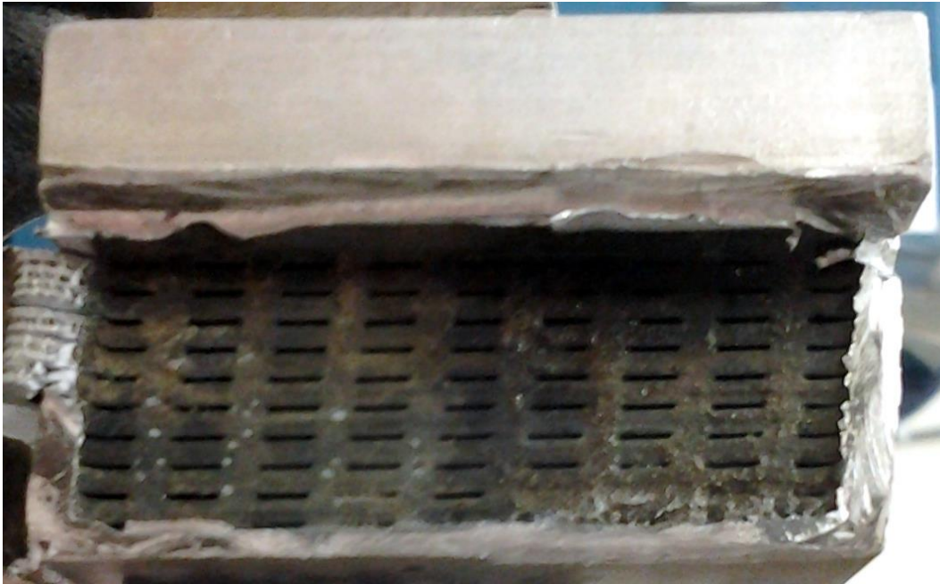
Figure 5-19 Evidence of deformation caused by machining stresses
