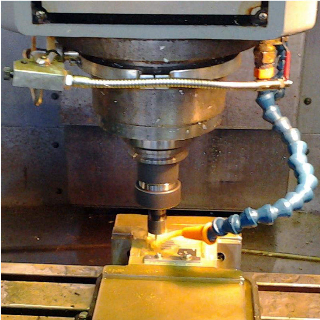
Figure 5-8 CNC milling of aluminum laminae
