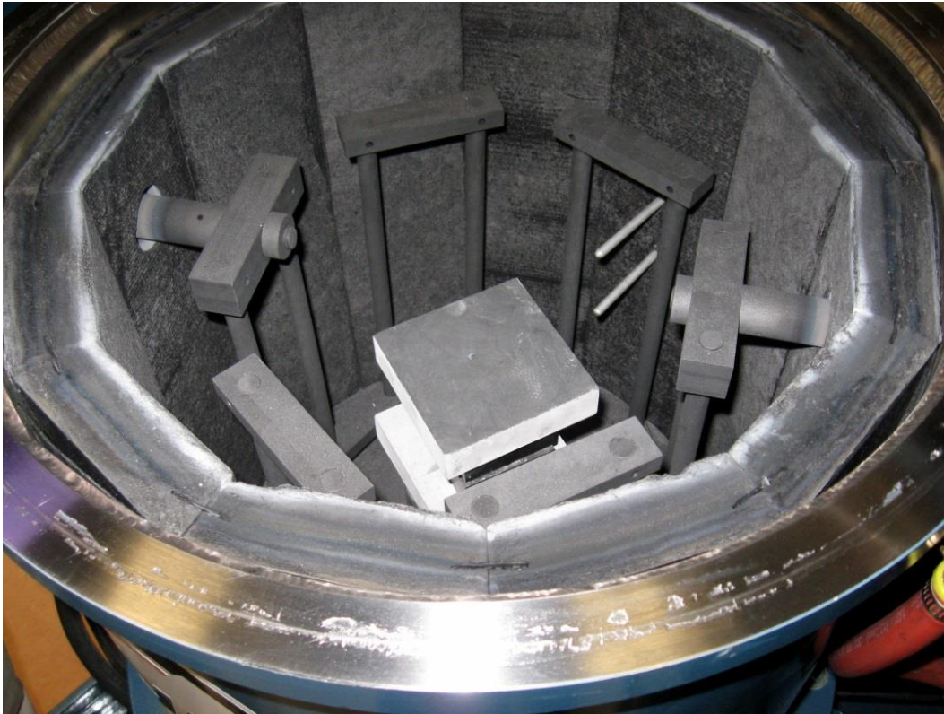
Figure 5-3 Interior view of the vacuum chamber of the vacuum hot press
