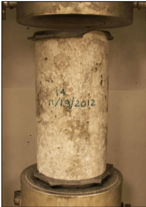
Figure E-2 (a) Geopolymer Concrete Mix (b) Plan View of Casted Cylinder (c) Failure Pattern on 3 Days Testing of Cylinder prepared from 1.29% CaO Fly ash of 14M concentration of Sodium Hydroxide Solution (Appendix B – Mix C4)
