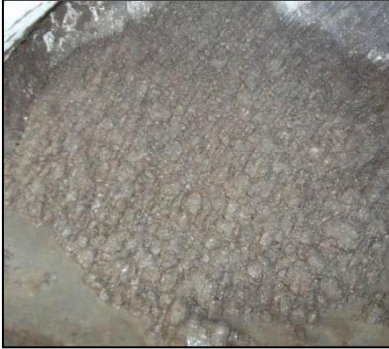
Figure 2-3 Geopolymer Mix with 5/8 aggregates
