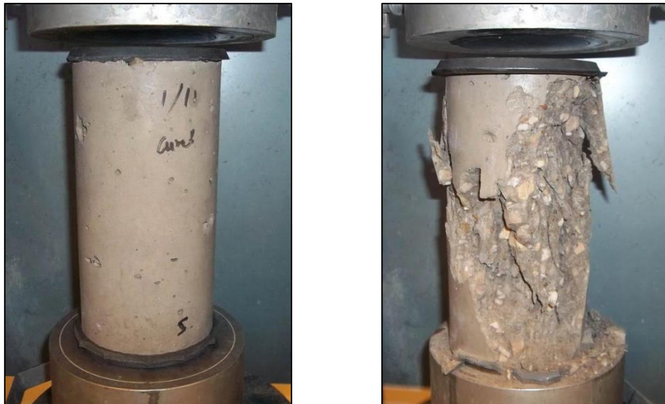
Figure 2-11 Failure pattern of Cylinder of 9.42% CaO Fly Ash
