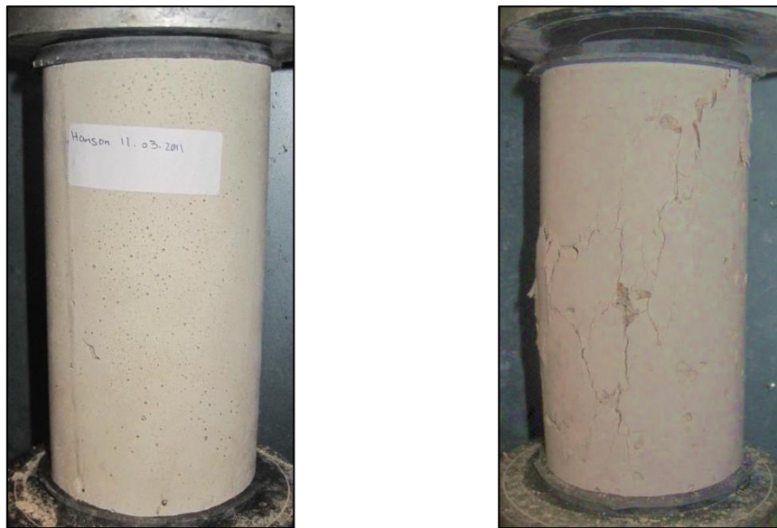
Figure 2-9 Failure pattern of Cylinder of 14.14% CaO Fly Ash
