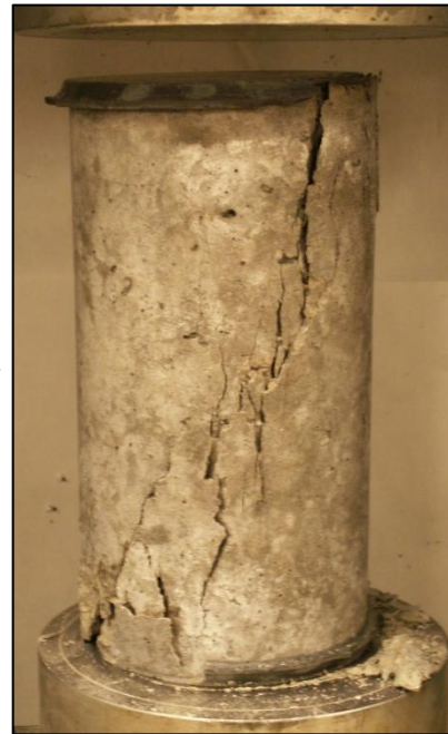
Figure E-1 (a) Geopolymer Concrete Mix (b) Plan View of Casted Cylinder (c) Failure Pattern on 1 Day Testing of Cylinder prepared from 1.29% CaO Fly ash of 8M concentration of Sodium Hydroxide Solution (Appendix B – Mix C3)
