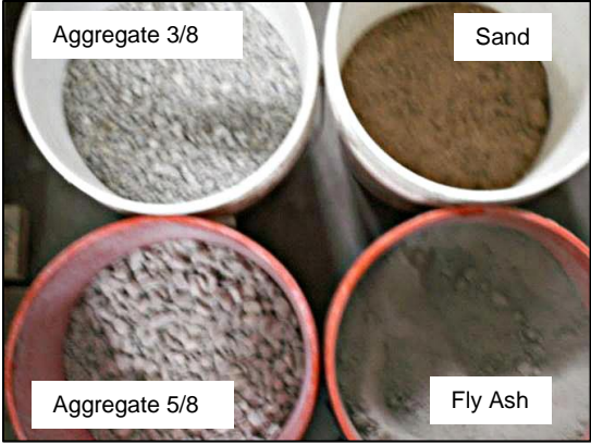
Figure 2-2 Constituents of Geopolymer
