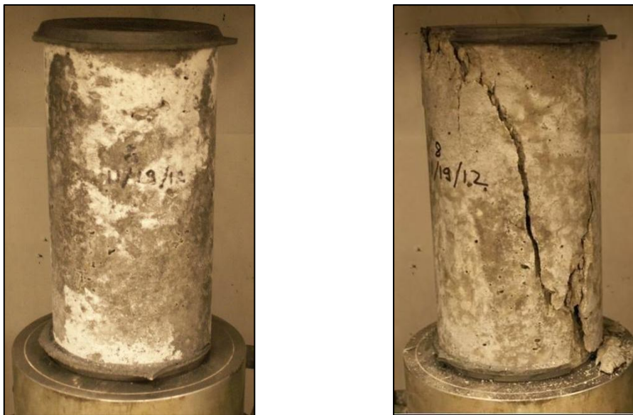
Figure 2-13 Failure pattern of Cylinder of 1.29% CaO Fly Ash
