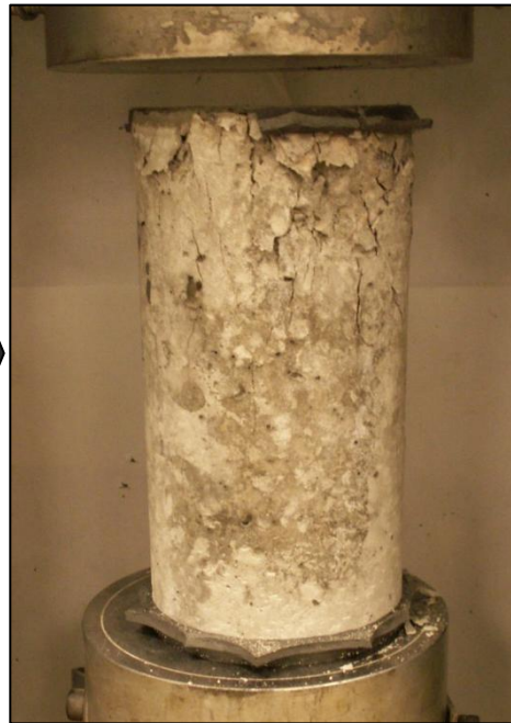
Figure E-2 (a) Geopolymer Concrete Mix (b) Plan View of Casted Cylinder (c) Failure Pattern on 3 Days Testing of Cylinder prepared from 1.29% CaO Fly ash of 14M concentration of Sodium Hydroxide Solution (Appendix B – Mix C4)
