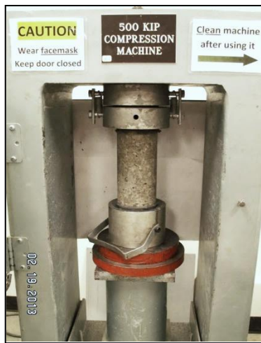
Figure 2-6 500 Kips Compressive Cylinder Testing Machine
