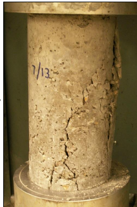
Figure E-4 (a) Geopolymer Concrete Mix (b) Plan View of Casted Cylinder (c) Failure Pattern on 3 Days Testing of Cylinder prepared from 9.42% CaO Fly ash containing Steel Fibers (Appendix B – Mix B36)
