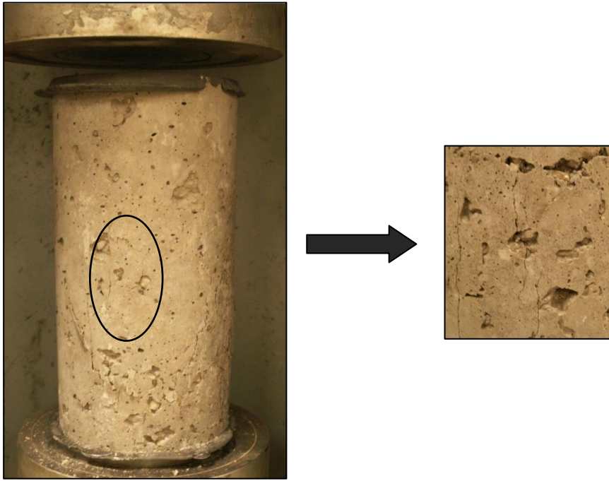
Figure E-5 Enlarged View of Failure Pattern on 28 Days Testing of Cylinder prepared from 9.42% CaO Fly ash containing Steel Fibers (Appendix B – Mix B36)
