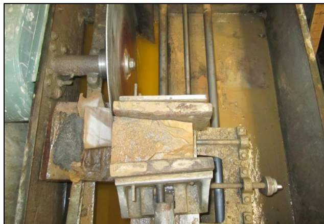
Figure 9 Kerosene Saw, Sample Position.
