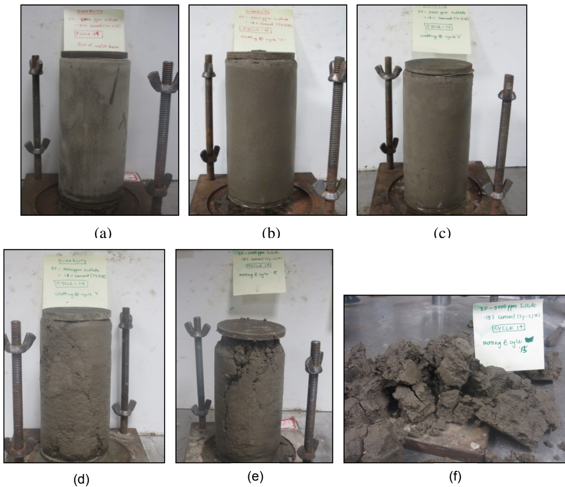
Figure 4.17 Pictures of EF-5000S 14-Cycle Sample showing Sample after (a) 28 days Curing, (b) 0-Cycle Wetting, (c) 3-Cycle Wetting, (d) 7-Cycle Wetting, (e) 12-Cycle Wetting and (f) 13-Cycle Wetting
