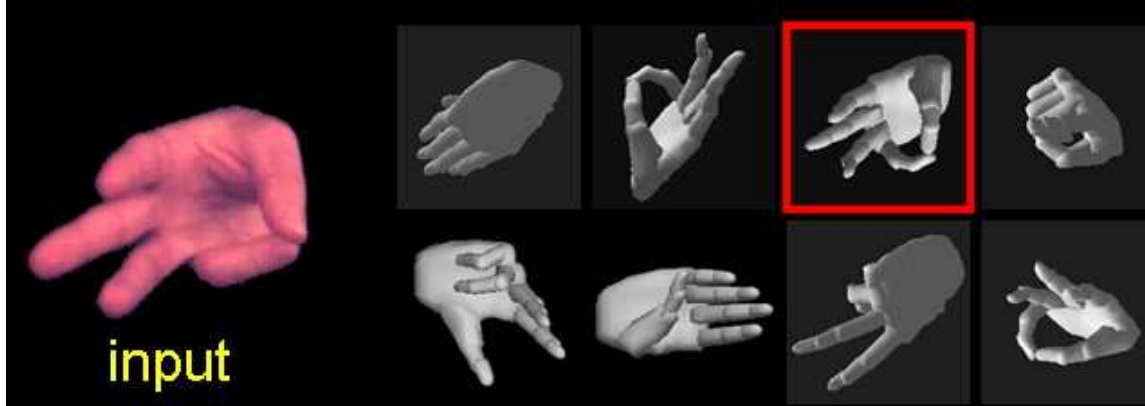
Figure 2.1. System input and output. Given the input image, the system goes through the database of synthetic images in order to identify the ones that are the most similar to the input image. Eight examples of database images are shown here, and the most similar one is enclosed in a red square. The database currently used contains more than 100,000 images.
