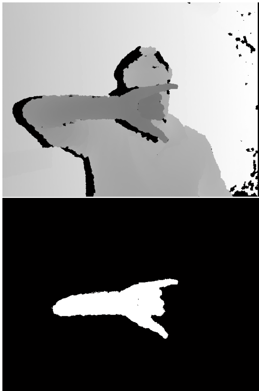
Figure 2.2. At the top image we can see the original depth image. At the bottom image we can see the segmented arm after performing depth segmentation using a rough estimation for an initial threshold. Original size for both images is 640 \times 480 .
