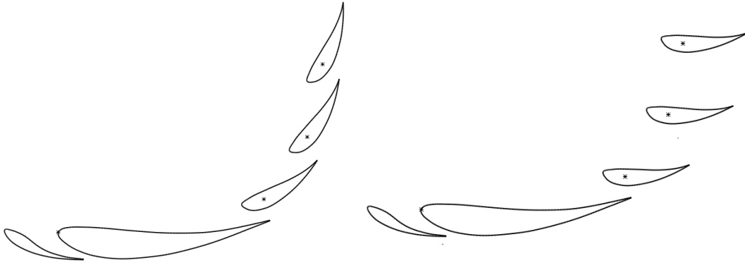
Figure 7. Multi-element wing in closed and open-position.
