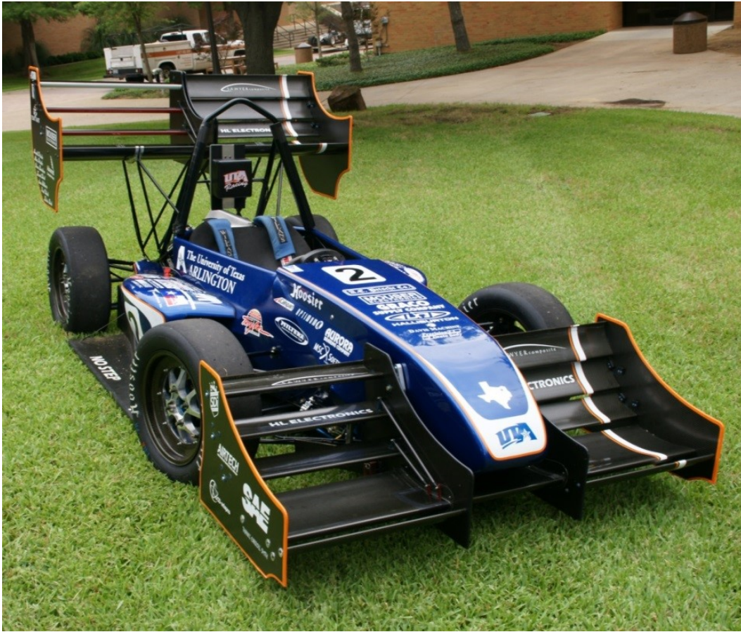
Figure 41. 2013 Formula SAE car with active aerodynamics.
