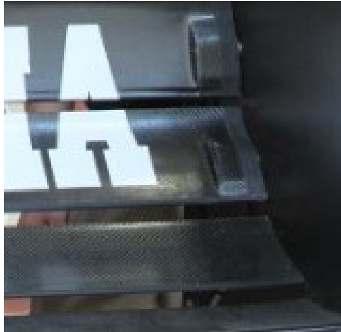
Figure 23. University of Oklahoma wing with servos embedded into wing elements.
