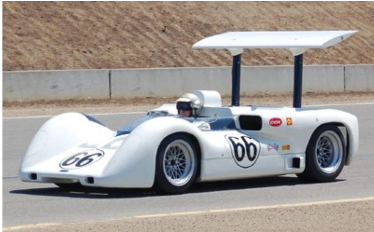
Figure 4. Chaparral 2E racecar with driver controlled rear wing [3].
