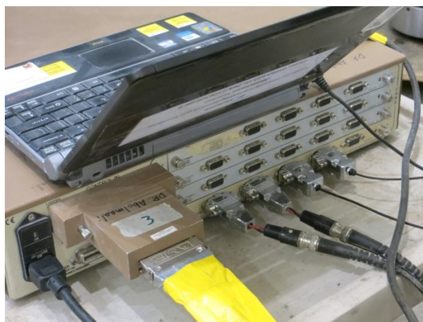
Figure 2-10 Sensors Connections to the Data Acquisition System
