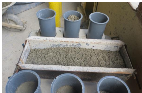
Figure 2-3 Beam and Cylinder Mold on the Vibrating Table
