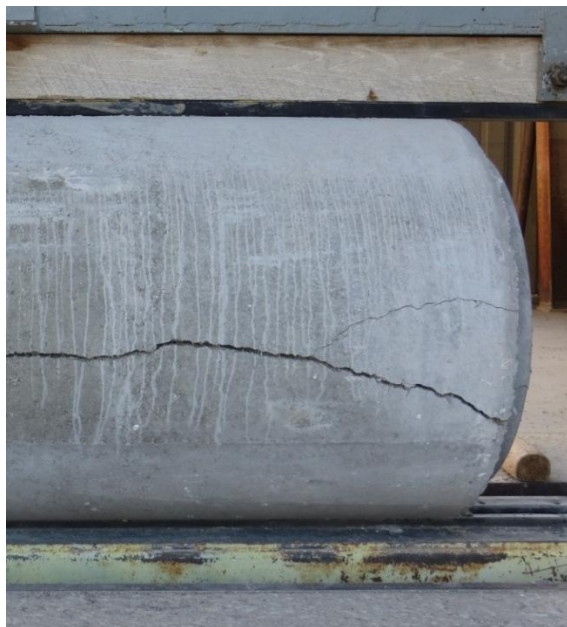
Figure 3-18 Secondary Crack Development
