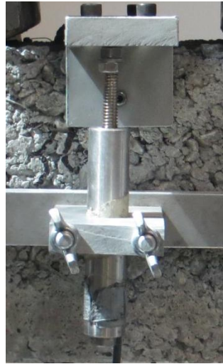
Figure 2-7 Linear Displacement Sensor (LVDT)
