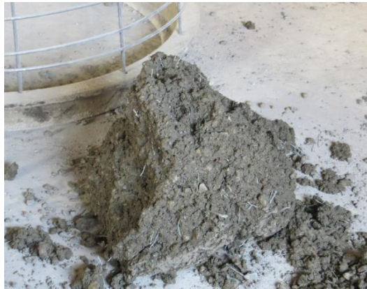
Figure 2-4 Solidified Dry Mix
