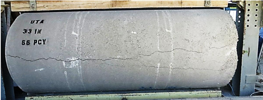
Figure 3-22 Multi Crack Development
