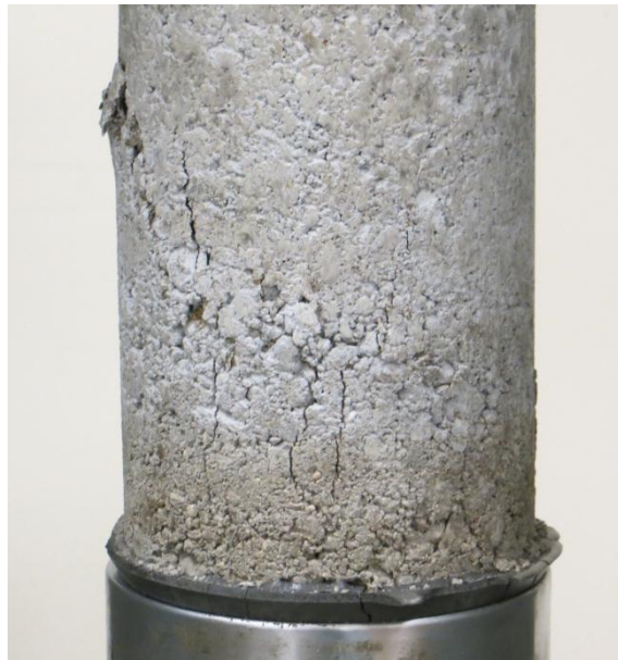
Figure 2-20 One Side Failure due to Poor Capping
