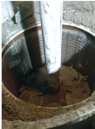
Figure 1-4 Packerhead Machine Rotors
