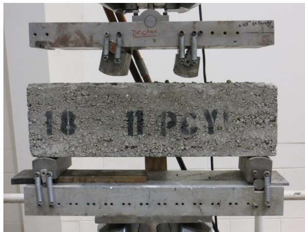
Figure 2-6 Support and Loading Steel Pads Arrangement
