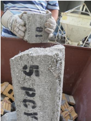
Figure 2-13 Brittle Failure of 5 lb/yd 3 steel fiber beam
