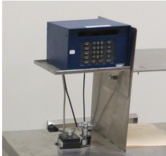
Figure 2-22 Load Display and Control Valve
