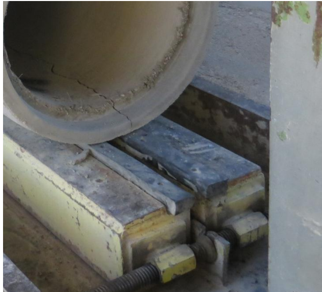
Figure 3-6 Lower Bearing Adjustment
