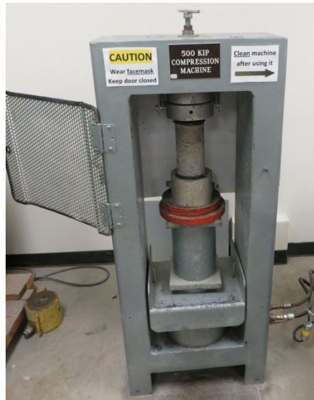
Figure 2-21 Compression Testing Machine
