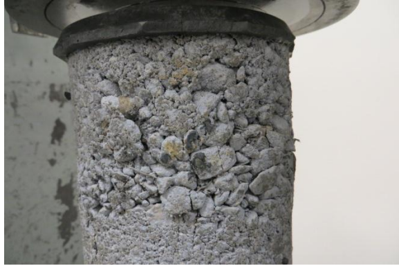
Figure 2-23 Segregation due to Dry Mix and High Frequency Vibration Consolidation
