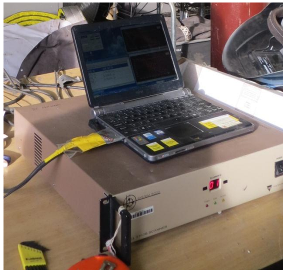
Figure 2-9 Data Acquisition System
