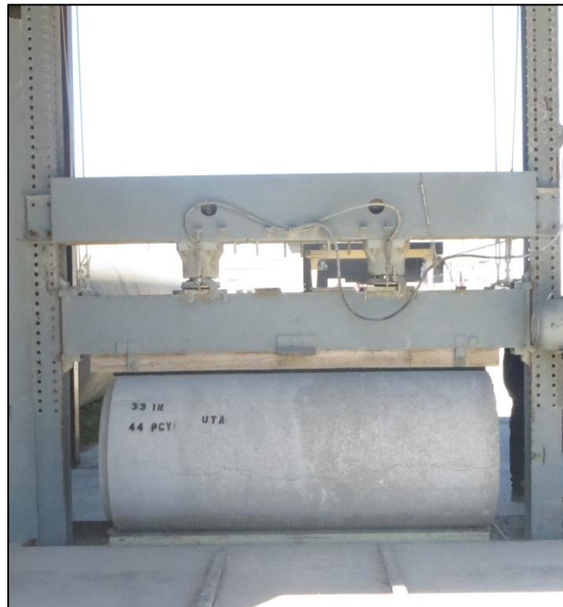
Figure 3-5 Three-Edge Bearing Test Machine
