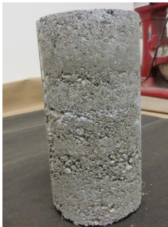
Figure 2-18 Layers of Concrete in a Compressive Cylinder Test Specimen due to Dry Mix
