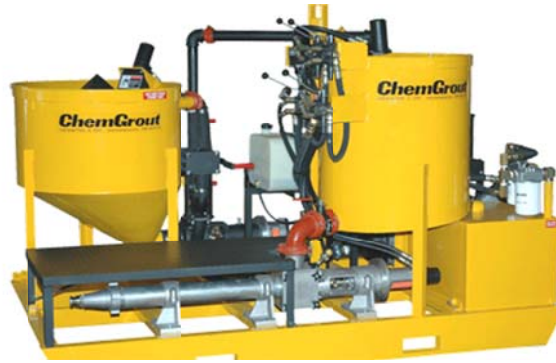
Figure 2-16 Grout mixer system used to on-site grout production ( www.chemgrout.com )
