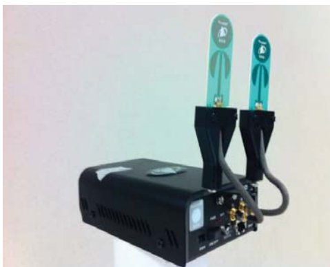
Figure 6.1. P220 in monostatic mode.
