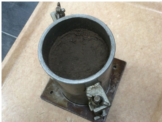
(c) Mold after compaction
