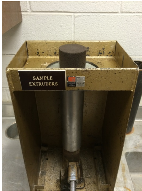
(c) Mold set up at the sample extruder
