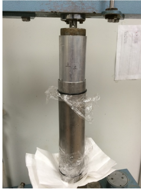
(b) Compaction process (five layers)
