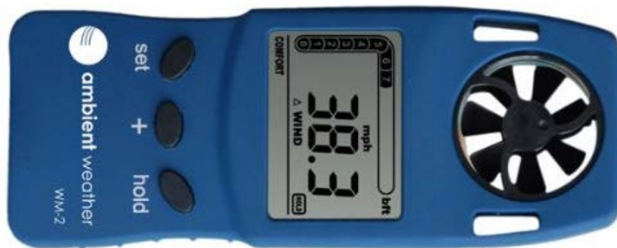
Figure 3.12 Anemometer for Monitoring Wind Speed and Direction in the Landfill
