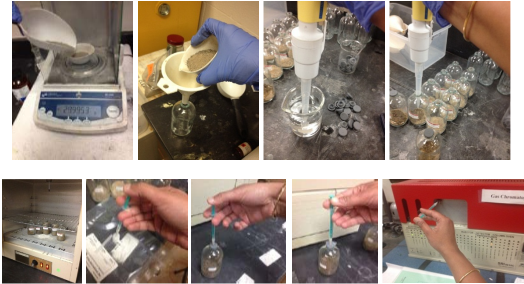
Figure 3.20 Batch Experiments/ Incubation in the Laboratory for Determining Methane Oxidation Capacity of the Soil
