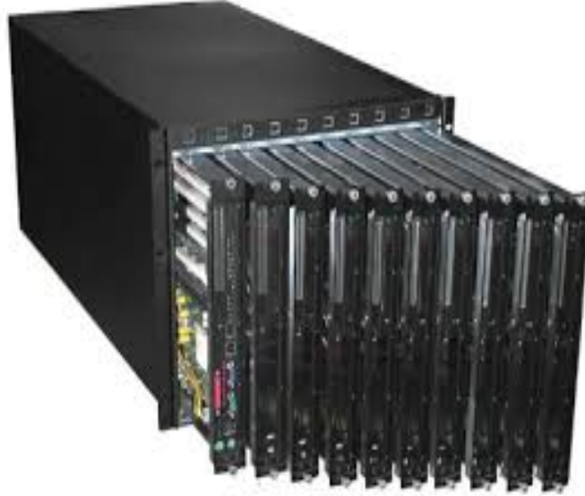
Figure 3.2. Blade server in chassis.
