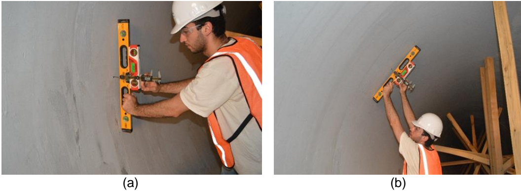
Figure 2-11 Mop-119 measurements taken per section at (a) 90 degree (b) 45 degree
