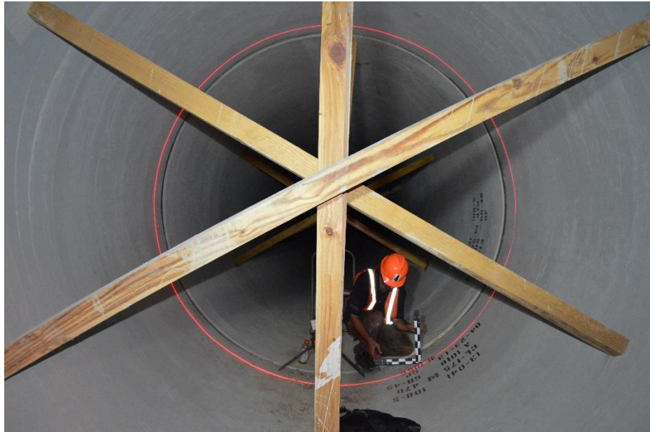
Figure 2-14 Laser photo profile method at start of pipe joint number 1066 at placement
