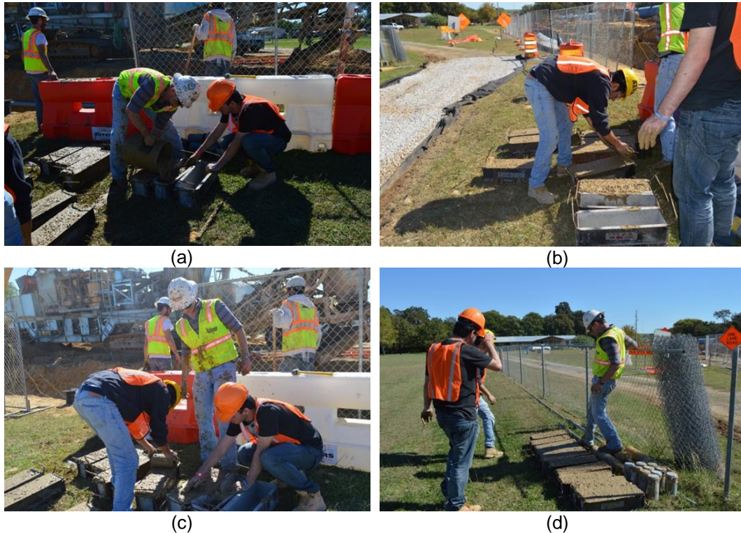
Figure 2-41 Casting procedure of CLSM beam and cylinder molds (a) pouring CLSM in mold (b) Filling mold with CLSM (c) Leveling surface for smoothness (d) Molds set for curing
