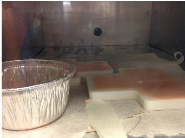
Figure 3-26 RTV silicone in 3D printed molds during degassing
