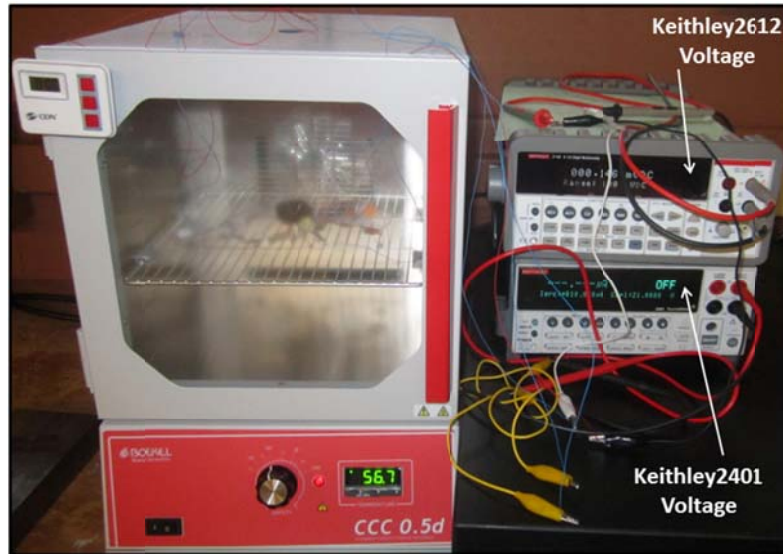
Figure 6.5 Image of the experimental setup for thermal calibration of temperature sensors on each die.
