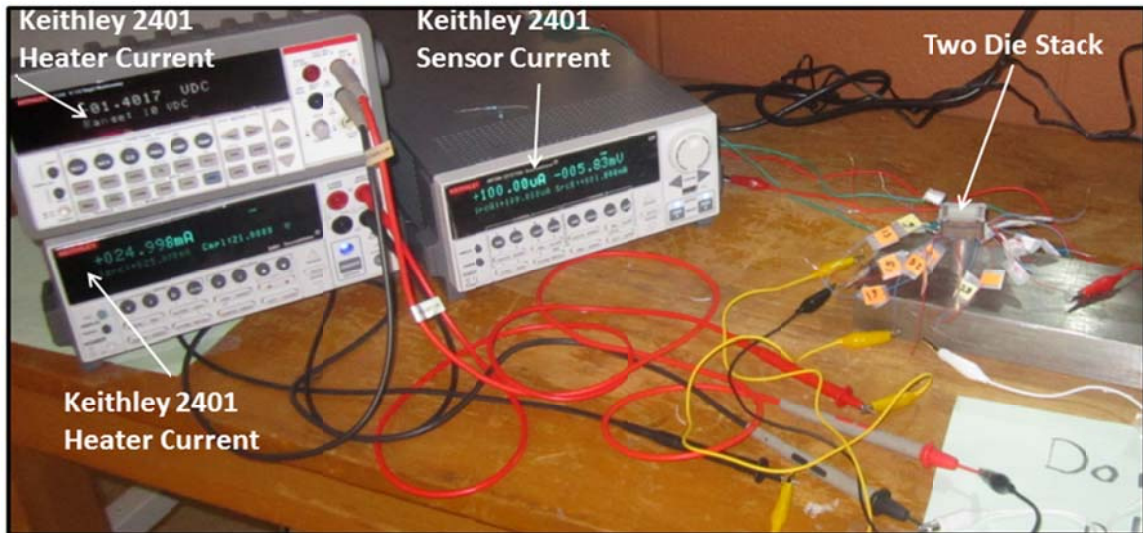
Figure 6.7 Experiment setup for studying heater effects on sensors.
