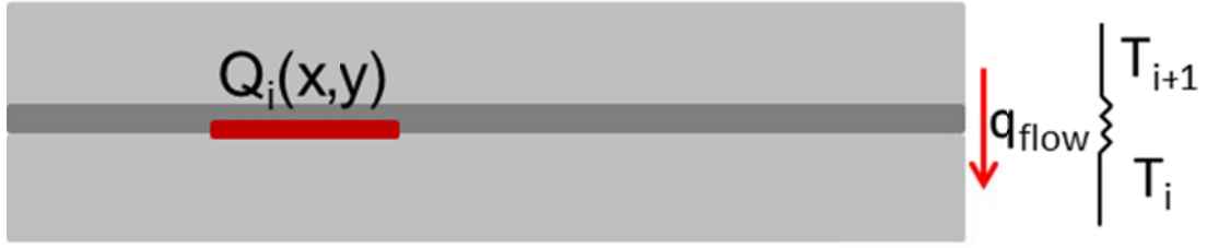
Figure 5.2 A model for thermal contact resistance between two adjacent die
