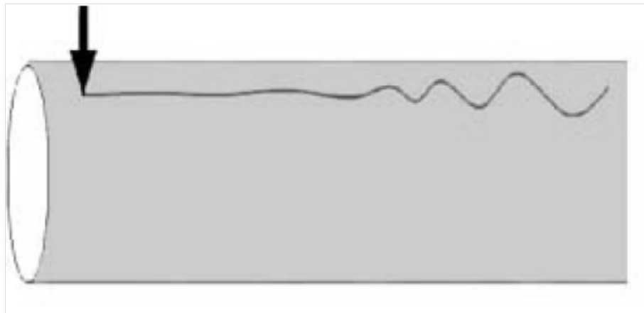
Figure 2.14 Rapid Crack Propagation (Adapted from Performance Pipe, 2012)
