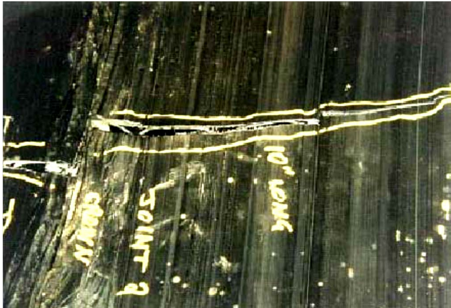
Figure 2.12 Macroscopic Brittle Failure of HDPE (Zhang, 2005)
