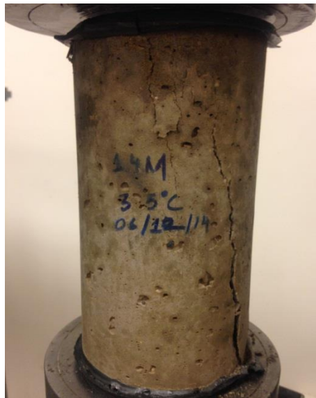
Figure 4-14 Failure Pattern of 14M NaOH Geopolymer with 9.42% flyash
