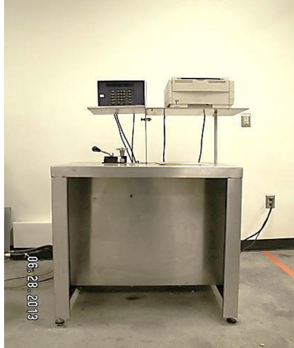
Figure 3-4 Control unit for mechanical tester
