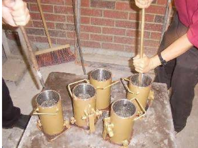
Figure 3-2 Compaction of geopolymer into cylindrical molds
