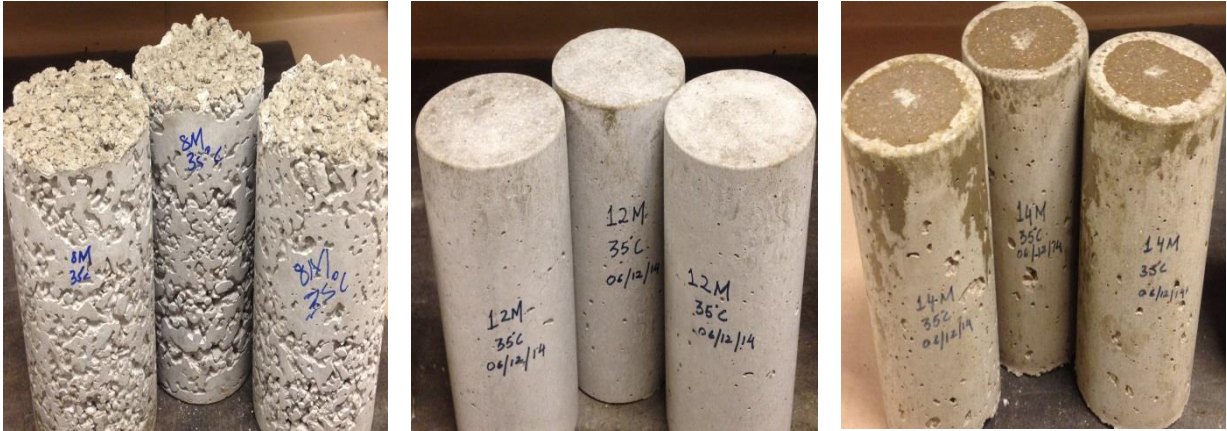
Figure 4-9 Cast Geopolymer Cylinders (a) 8 M (b)12 M and (c) 14 M NaOH geopolymer all with 9.42% CaO
