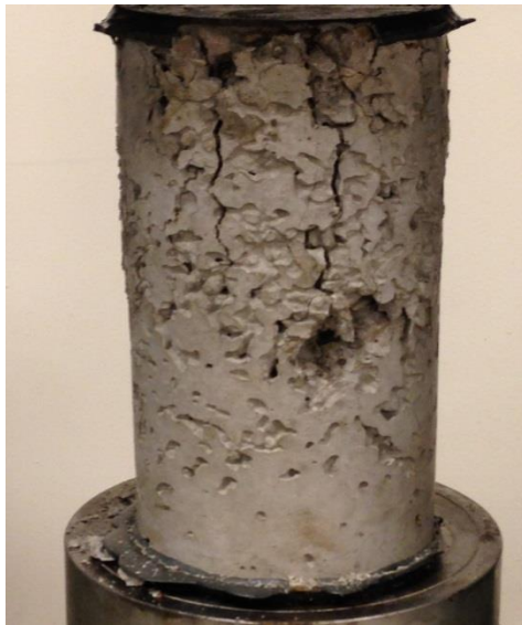
Figure 4-10 Failure Pattern of 8M NaOH Geopolymer with 9.42% CaO flyash.
