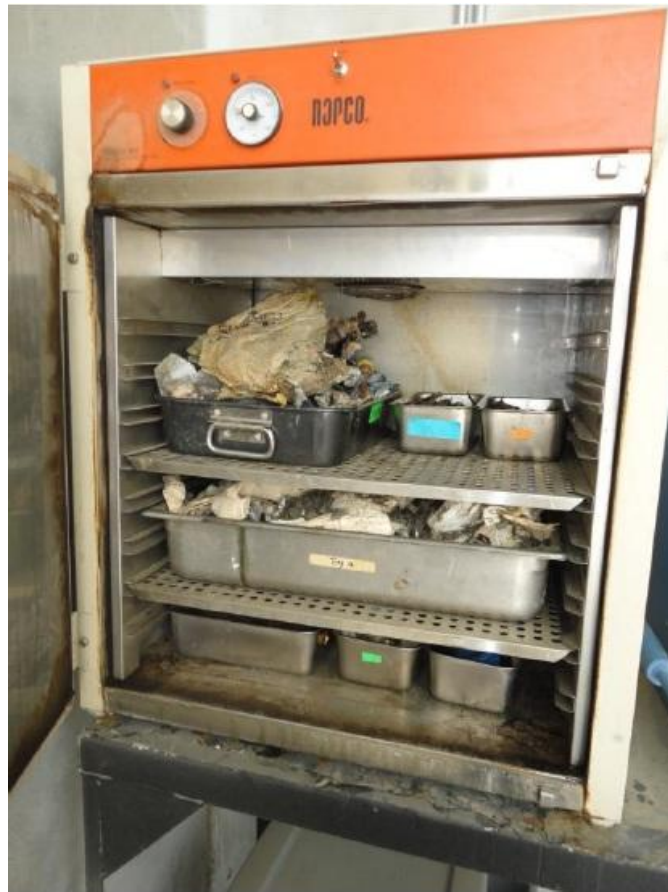
Figure 3.6 Drying the Samples for Moisture Content Test
