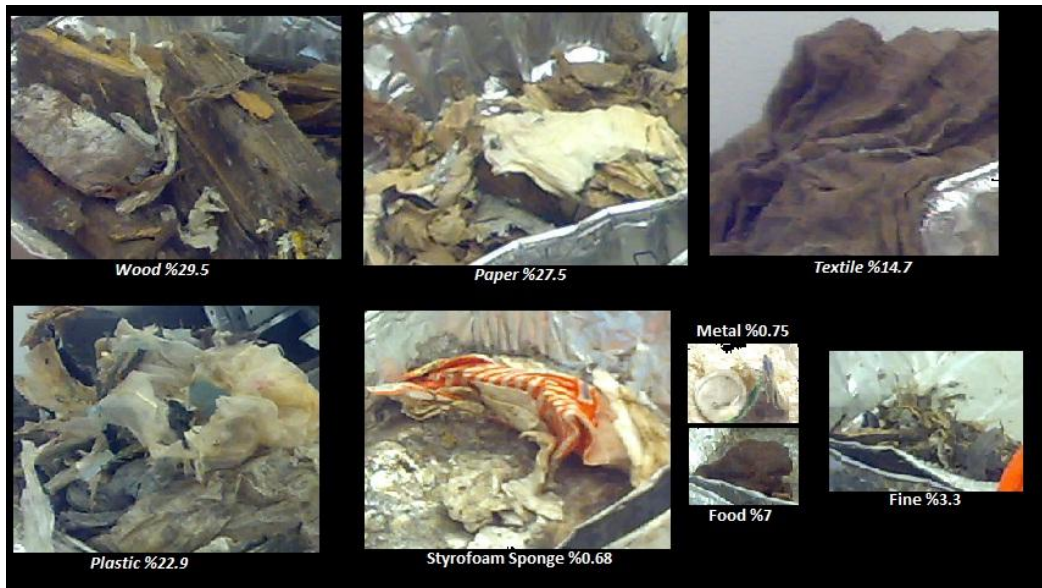
Figure 3.5 Separation of an MSW mass to its constituents
