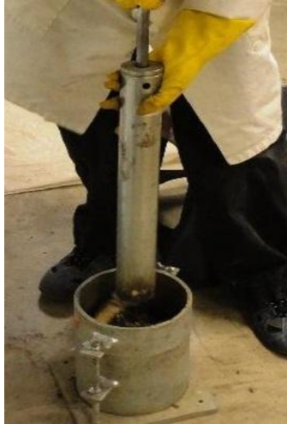
Figure 3.7 Applying the standard proctor compaction effort
