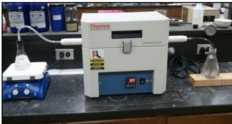
Figure 3.4: Experimental set-up of the heat treatment
