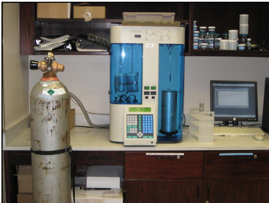
Figure 3.10: Experimental set-up of the surface area analyzer
