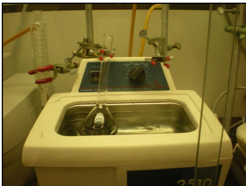
Figure 3.5: Experimental set up of the nitric acid treatment
