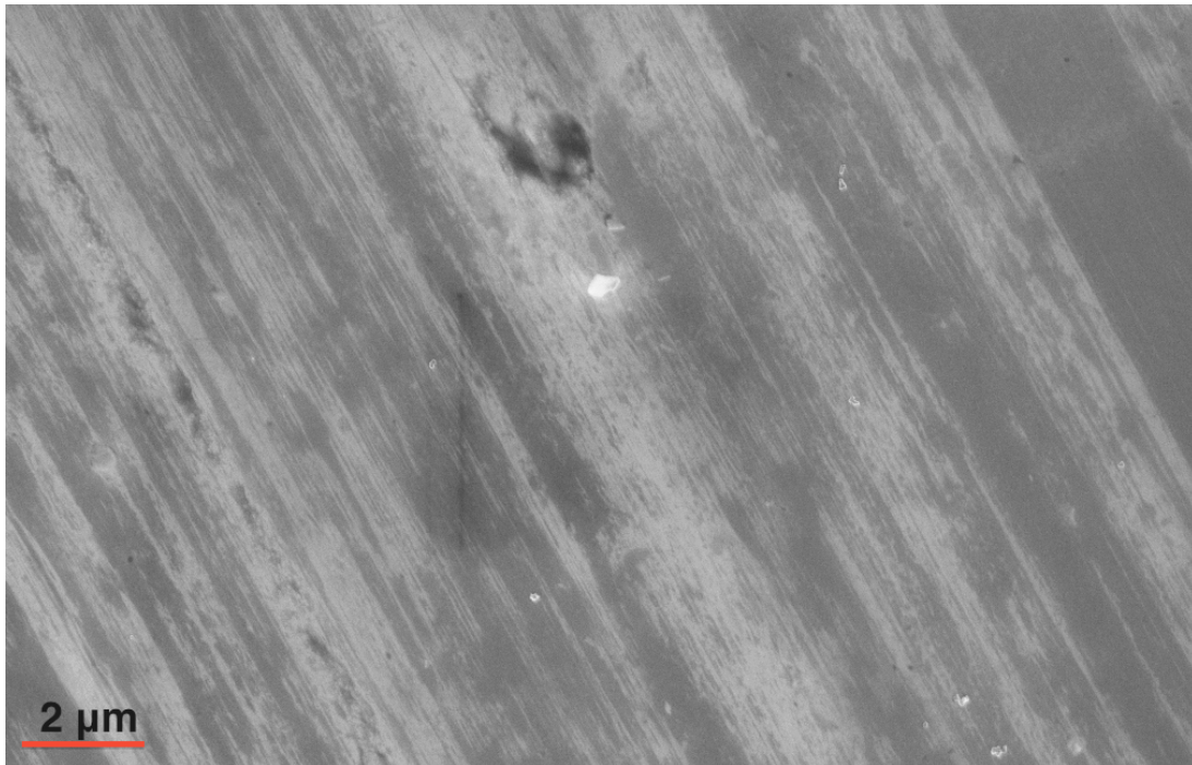
Figure 5.3 Scanning electron microscope image of the wear scar formed on the stationary four ball by test formulation A that had {Mineral Oil + 0.1 wt % P ZDDP + 5% dispersant}
