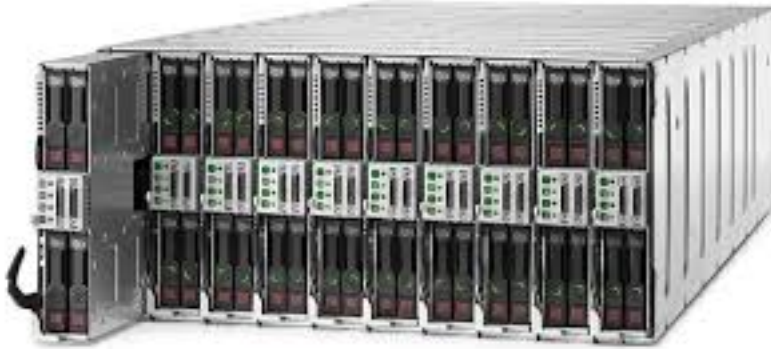
Figure 1-3: A server sled with multiple servers on board
