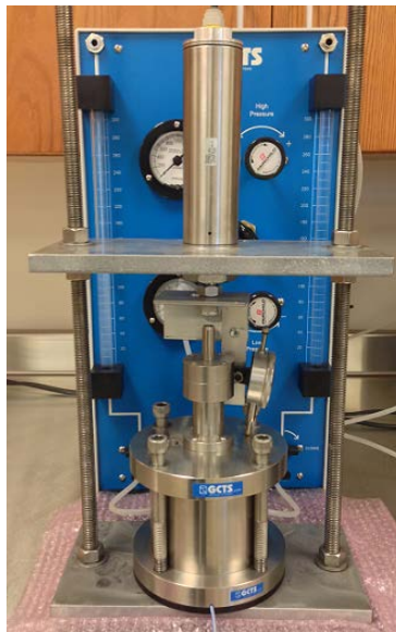
Figure 3.7 Fredlund's device (Tempe cell) for SWCC measurements
