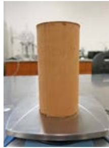
Figure 4.6 Desiccated specimen after RH application ( s = 300 MPa)
