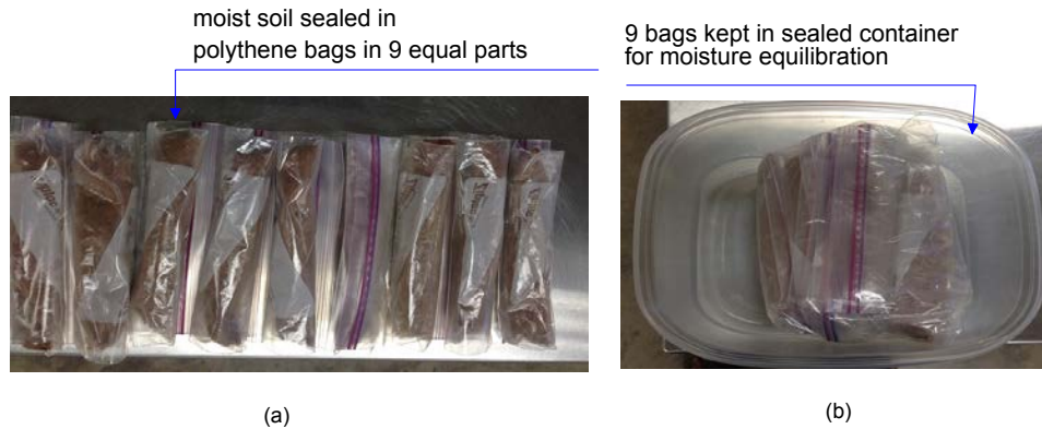
Figure 3.4 Soil storage for moisture equilibration prior to compaction
