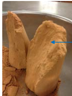
Figure 4.12 Particle crushing along failure planes from CD100-20 MPa test
