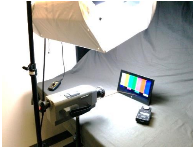
Figure 5-8 Measurement of display contrast ratio
