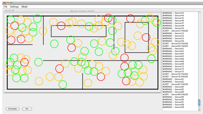
Figure 4-10: Monitoring mode of SPSM, where green means the sensor is fine, yellow that there is a warning and red that the sensor is faulty.
