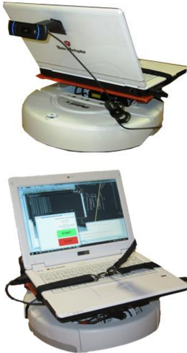
Figure 4-1: eyeDog, the prototype assistive-guide robot.
