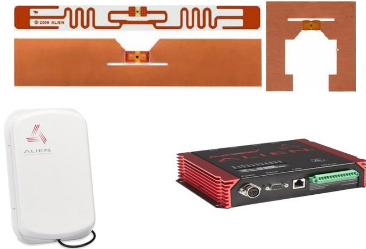
Figure 3-2: The RFID equipment used including different designs of Alien RFID Tags (top) and receiver, antenna (bottom).
