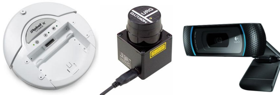
Figure 4-2: The hardware components of the eyeDog: the iRobot platform (left), Hokuyo LIDAR (middle) and Logitech webcam (right).
