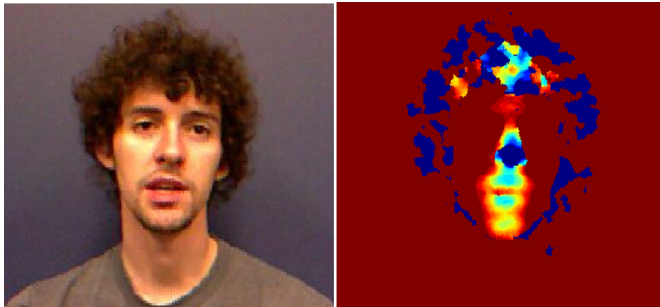
Figure 2-9: Example of a collected color video frame (left) and the corresponding depth frame (right).
