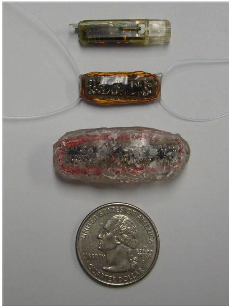
Figure 1.2 The 2 nd generation of the GERD sensor that is a single sensor detector (second from the top) is in a very compatible size with the Bravo (Top), The 3 rd generation (second from the bottom) equipped with the two sensors. Both are batteryless operated.
