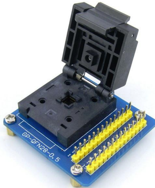
Figure 5.2 A socket for the package of QFN28 (5x5) [64]
